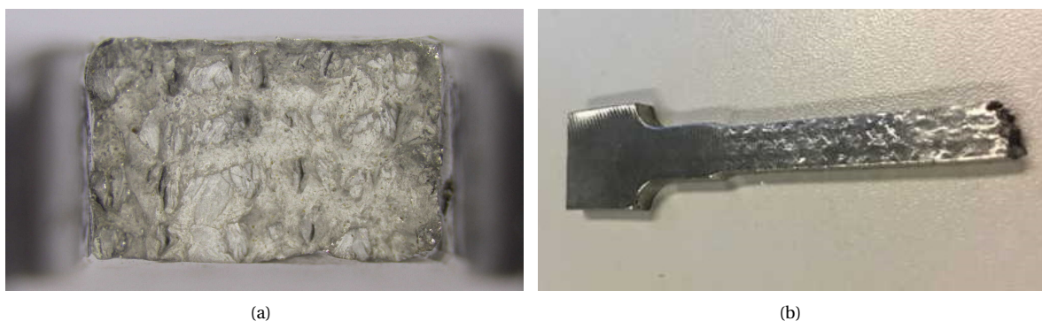
Figure 4.17: (a) Fracture surface and outer surface (b) of a tensile specimen built with the adjusted shielding gas flow rate of 20 l/min.
