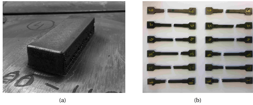
Figure 4.11: (a) Deposited multilayer structure of Inconel 718 using a crosswise deposition and (b) the tensile test specimens after testing.
