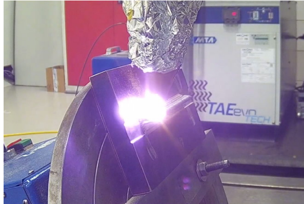
Figure 4.27: Setup during deposition of the hard flank material, the substrate is placed on a 20° tilted table to achieve a perpendicular deposition.
