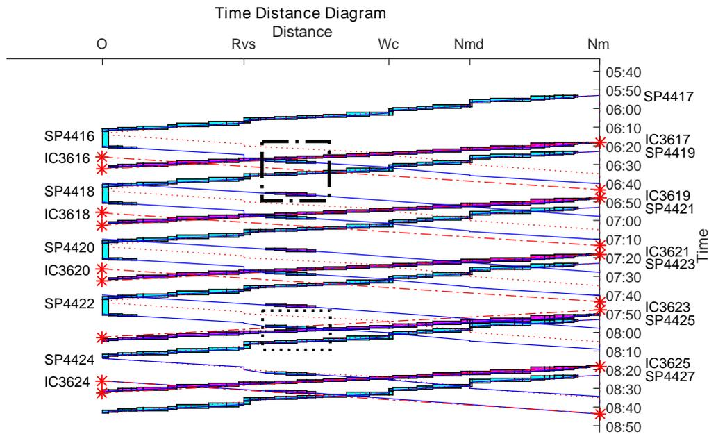
Figure 2.7: Blocking time diagram when the disruption starts at 6:00 with IC3622 cancelled
