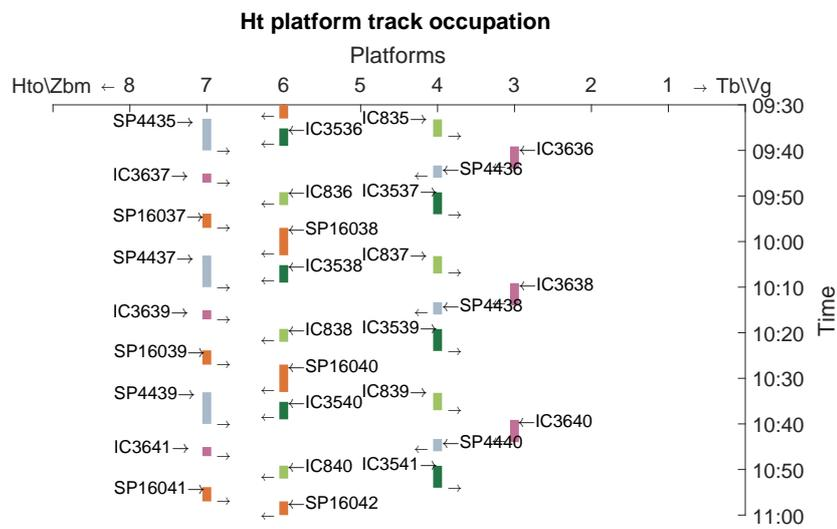
Figure 5.10: The result for the platform track occupation of the original timetable in the secondary short-turning station, Ht.
