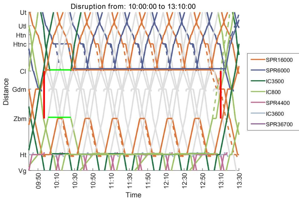
Figure 4.18: Optimal short-turning solution for disruption from 10:00 to 13:10.
