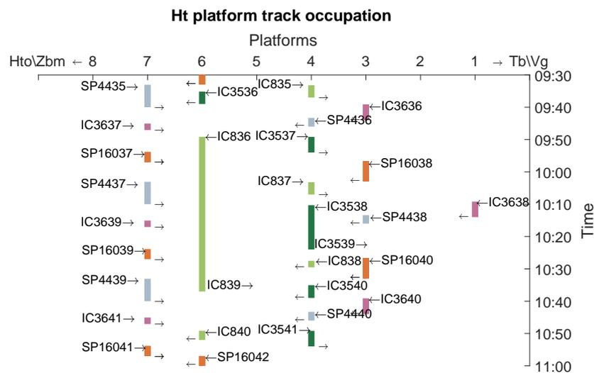
Figure 5.11: The rescheduled platform track occupation in the secondary short-turning station, Ht.
