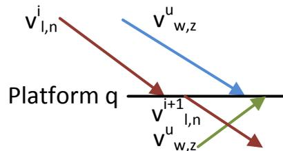
Figure 4.8: The platform occupation constraint for the non short-turning services.
