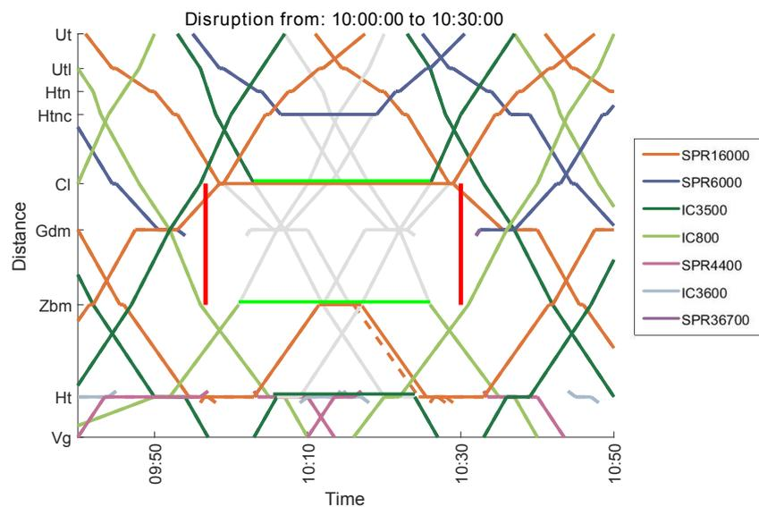
Figure 4.12: Optimal short-turning solution for disruption from 10:00 to 10:30.
