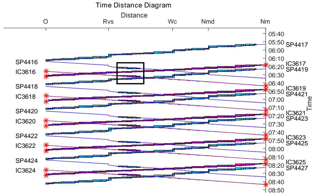
Figure 2.5: Blocking time diagram of the original timetable
