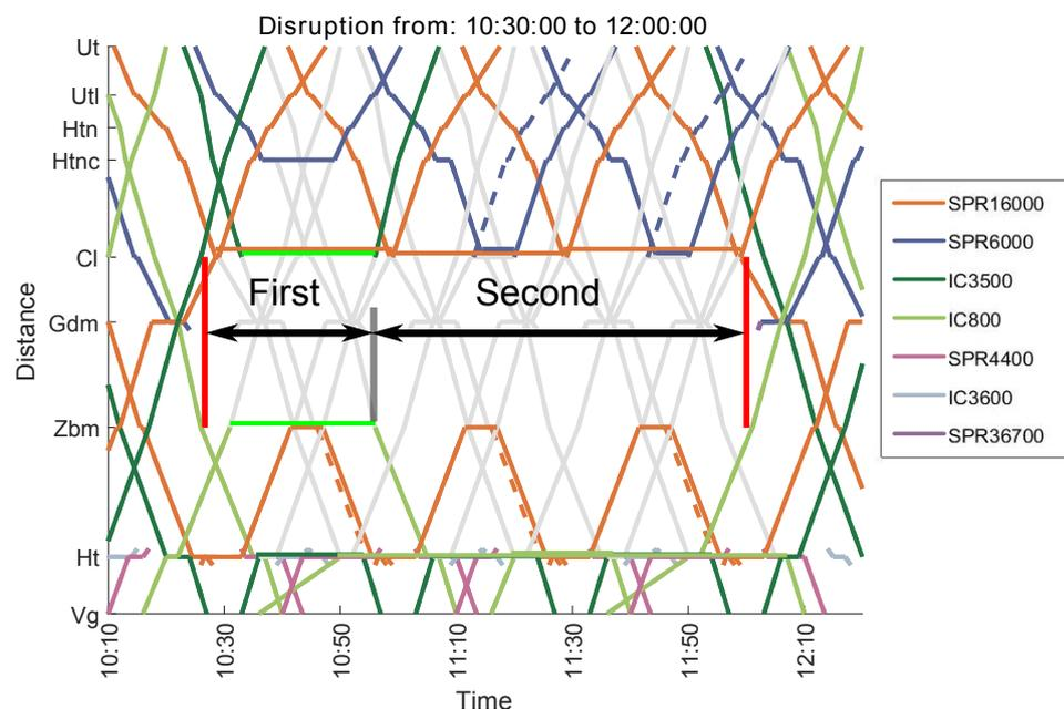
Figure 4.15: Optimal short-turning solution for disruption from 10:30 to 12:00.
