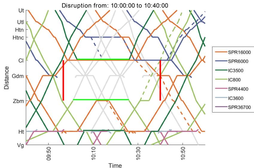
Figure 4.13: Optimal short-turning solution for disruption from 10:00 to 10:40.
