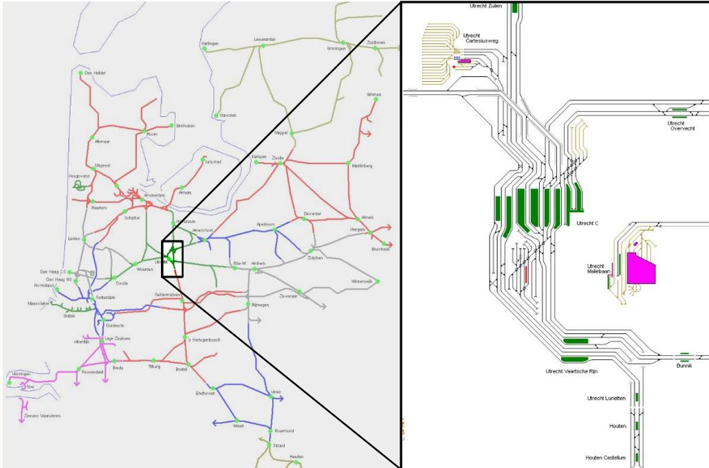
Figure 1.6: The macroscopic and microscopic representation of the Dutch railway network. Source: <http://www.sporenplan.nl/> (accessed September 25, 2017)
