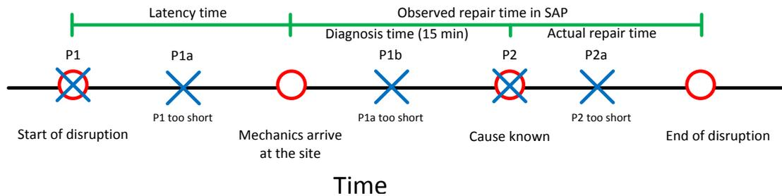
Figure 6.9: The time diagram of a railway disruption
