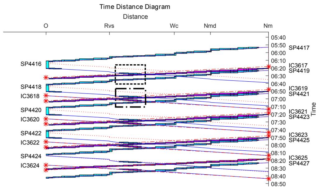
Figure 2.6: Blocking time diagram when the disruption starts at 6:00 with IC3616 cancelled
