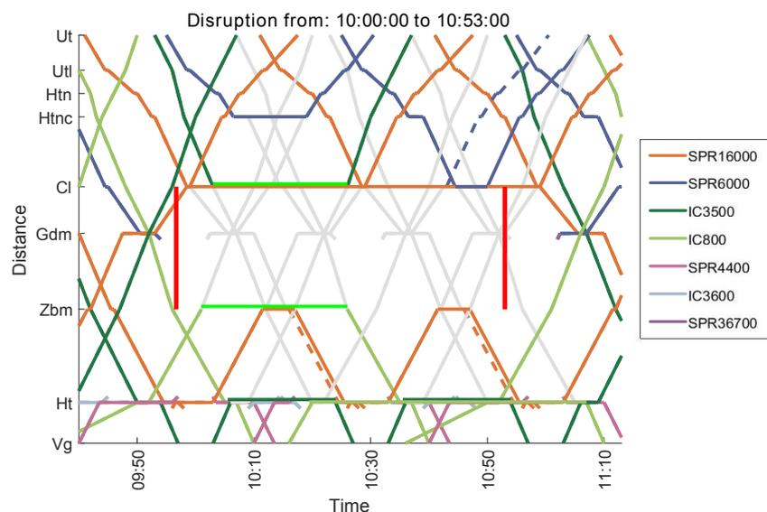
Figure 4.14: Optimal short-turning solution for disruption from 10:00 to 10:53.
