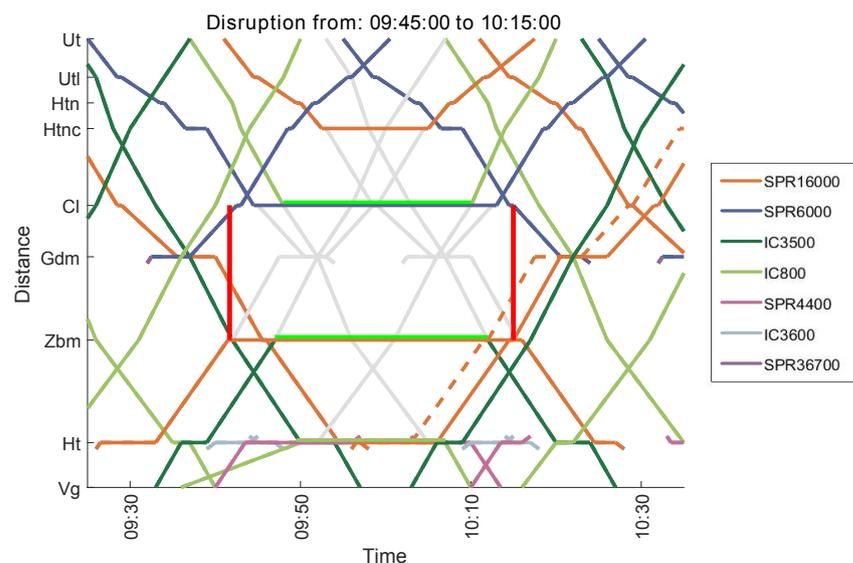
Figure 4.11: Optimal short-turning solution for disruption from 9:45 to 10:15.
