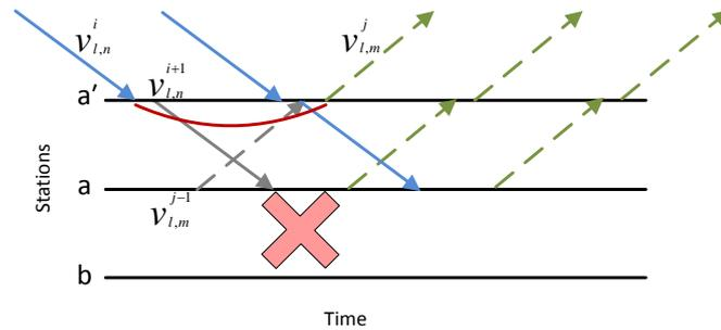
Figure 6.5: The cancellation resulting from short-turning in station  $a'$
