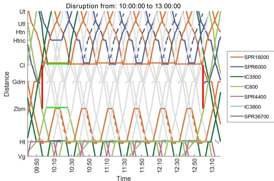
Figure 4.17: Optimal short-turning solution for disruption from 10:00 to 13:00.
