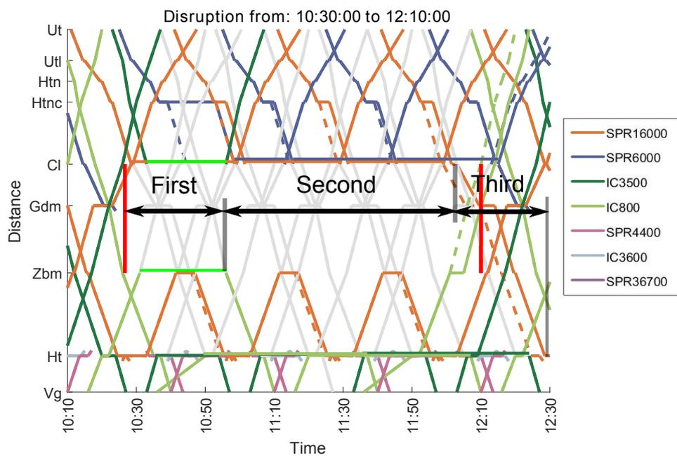
Figure 4.16: Optimal short-turning solution for disruption from 10:30 to 12:10.
