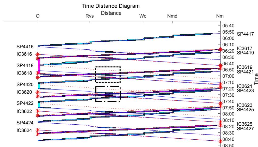
Figure 2.8: Blocking time diagram when the disruption starts at 6:30 with IC3617 short-turning on the upper track
