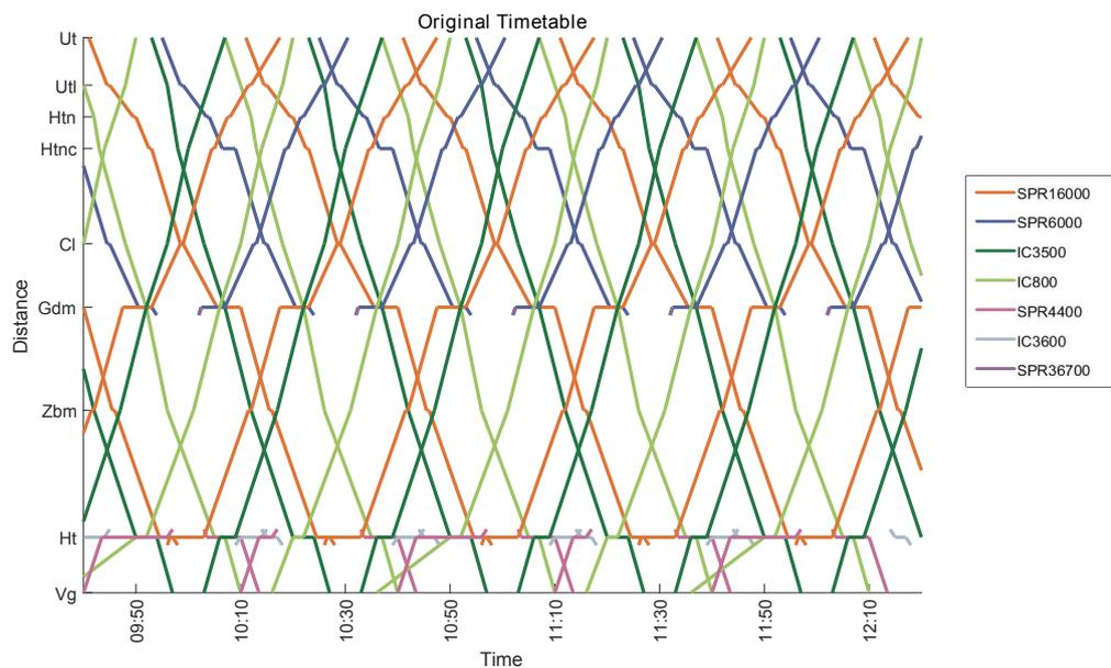
Figure 4.10: The time-distance diagram of the original timetable.
