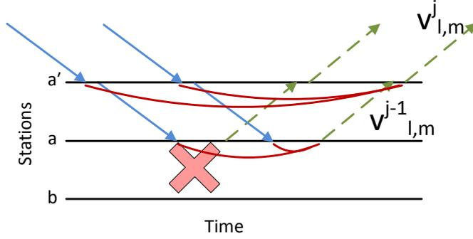
Figure 3.6: The short-turning options for services  $v_{l,m}^{j-1}$  and  $v_{l,m}^j$ .
