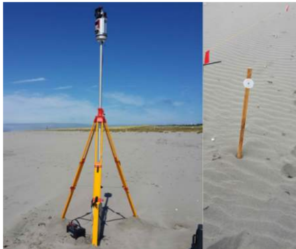
Figure 2.2: TLS set-up is shown on the left, TLS with camera on top on tripod. One ground control point is shown on the right.
