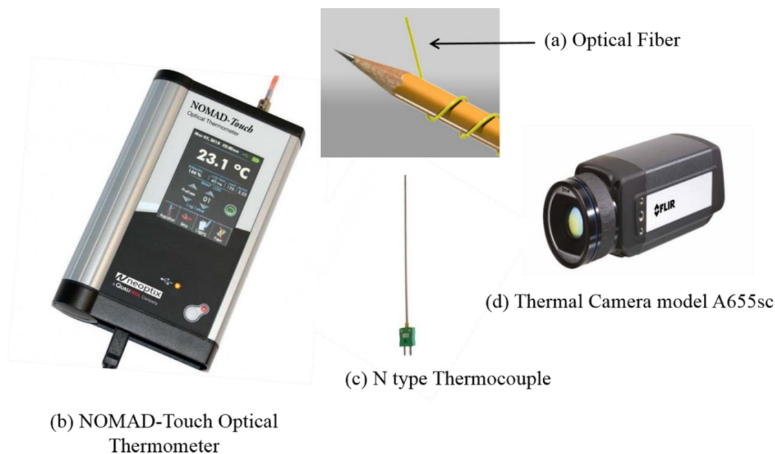
Figure 2.6 Temperature measurement techniques used: (a) optical fiber, (b) NOMAD-Touch optical thermometer, (c) N-type thermocouple and (d) thermal camera mode A655sc.
