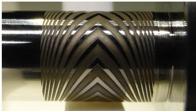
Figure 3.25: Herringbone grooved journal bearing of EPFL.[4]
