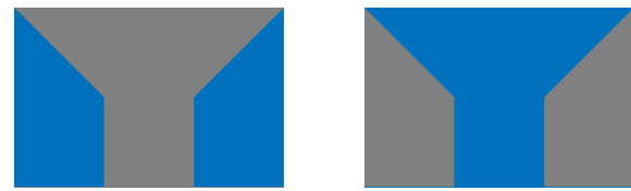
(a) Printable design, with a 45^\circ overhang angle (b) Drainable design, with a 45^\circ runoff angle
