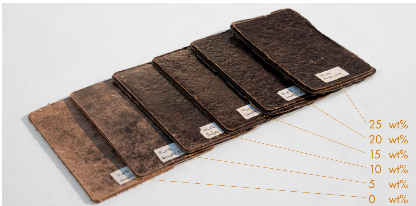
Figure 44. Hot-pressed plates from the material trial of moisture content variation
