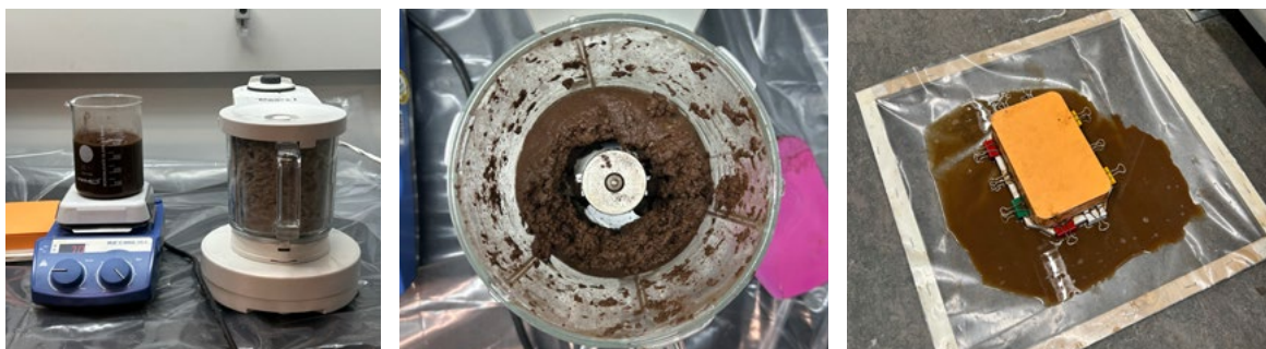
Figure 43. Mixing steps following the “wet”-process and the loss of lignin during the pre-compacting step.
