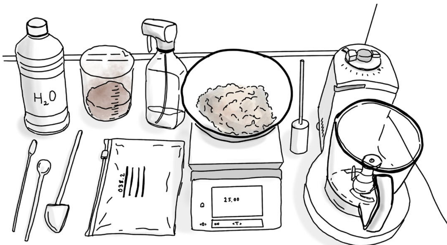
Figure 31. Drawing of mixture preparation setup, showing what equipment is required. Mixing is inside a dust extractor hood at H&T Lab
