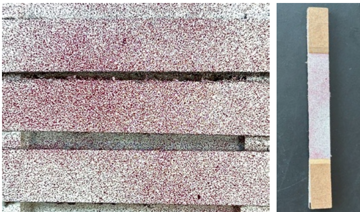
Figure 42. Close-up and total image of specimen with speckle pattern.
