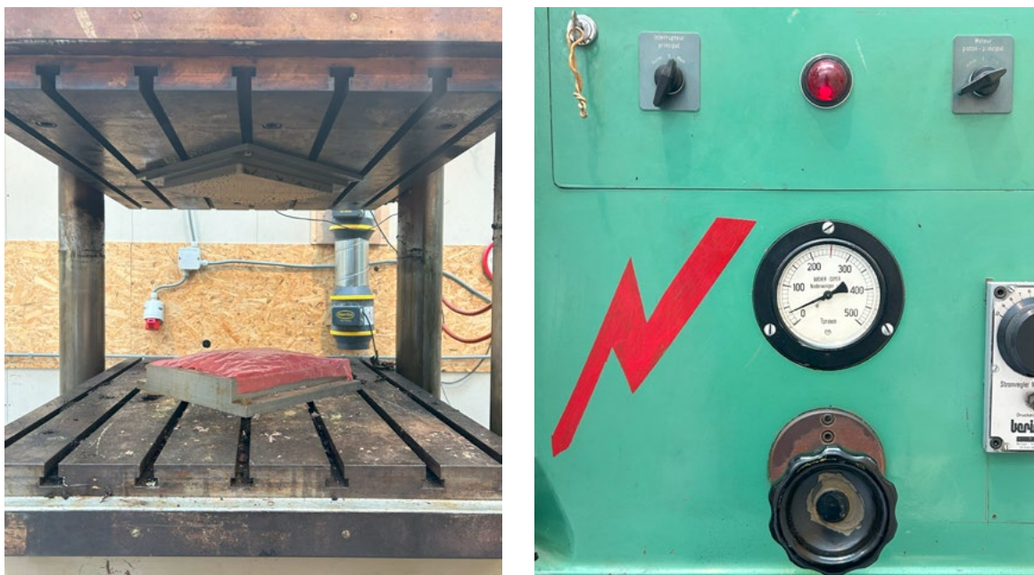
Figure 57. Industrial Type Hot-press at NPSP, showing the mould fixed in the press (left) and pressure gauge (right)
