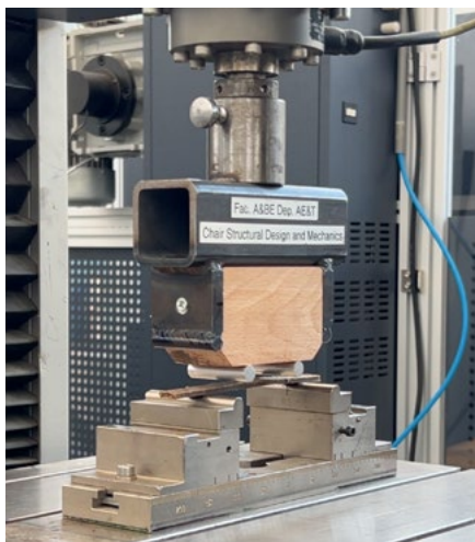
Figure 61. Photograph of 4-point bending test setup and of the deformed samples (C/L ratio trial) after testing.
