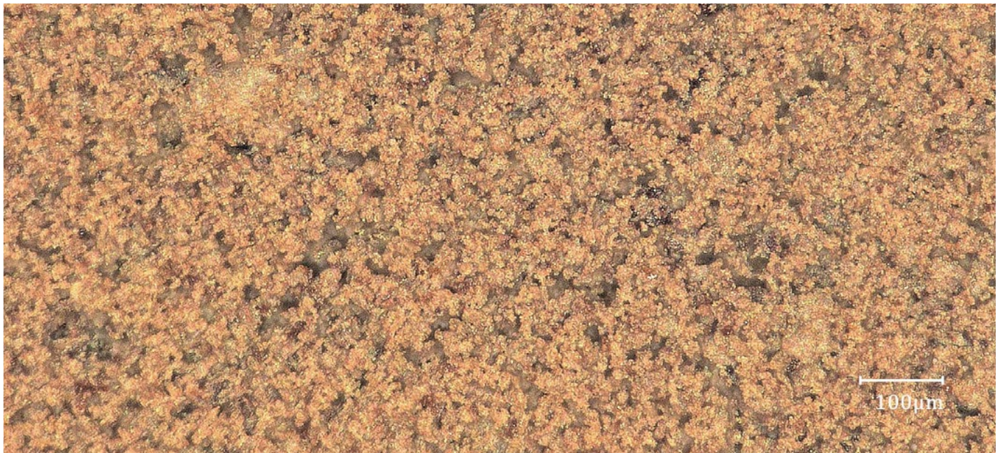
Figure 26. Image of Organosolv Lignin under Microscope with x250 magnification
