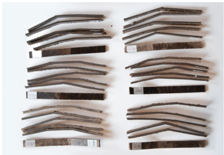
Figure 61. Photograph of 4-point bending test setup and of the deformed samples (C/L ratio trial) after testing.
