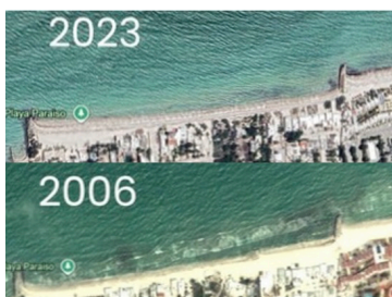
Figure 3.26: Large scale groin in Chelem (Google Earth, 2025)
