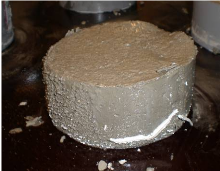
Figure 6-13: Removing of the mould 45 minutes after pouring.
