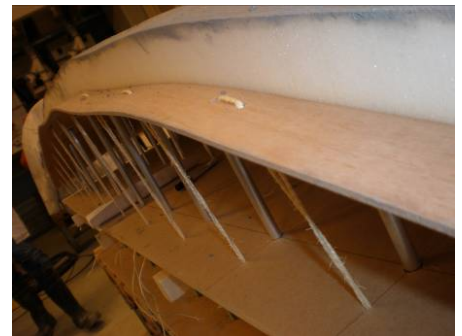
Figure 10-16: Buckling of the edge
