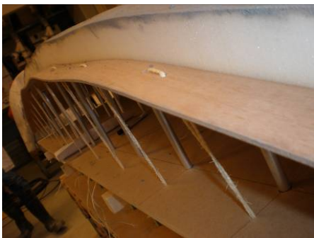
Figure 12: Buckling of the edge at the plate surface
