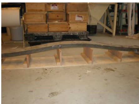
Figure 8-20: Demoulded element on the supports
