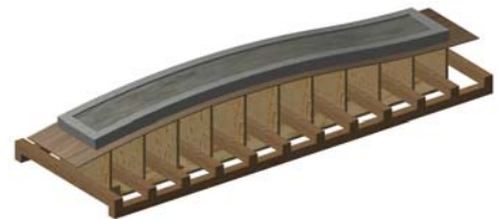
Figure 8-2: Deformed mould and concrete
