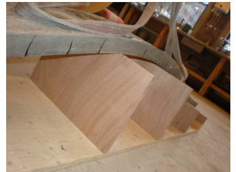
Figure 8-40: Demoulded element at the supports
