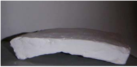
Figure 2-24: Element produced by M. Roosbroeck on a pin bed mould [21]
