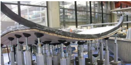
Figure 2-25: Actuator mould tested by K. Huyghe and A. Schoofs [9]
