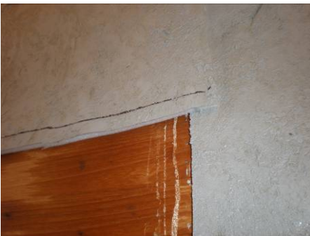
Figure 10-35: Stretched bottom layer of polyether after the first test
