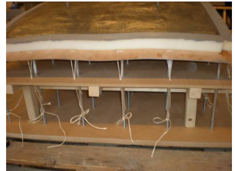
Figure 10-15: Edge after tensioning
