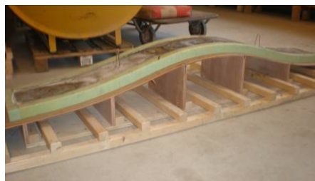
Figure 8-36: Deformed element in the formwork at the supports
