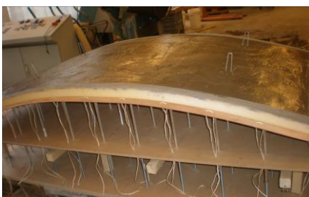
Figure 10-12: Just deformed element no cracks are visible
