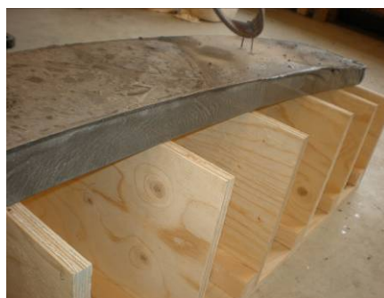
Figure 8-14: Demoulded element at the supports
