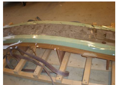
Figure 8-19: Deformed element after one day of hardening
