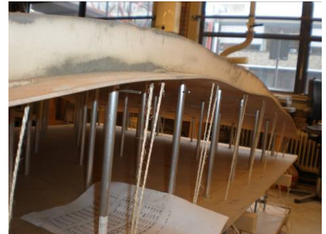
Figure 10-17: Buckling of the edge
