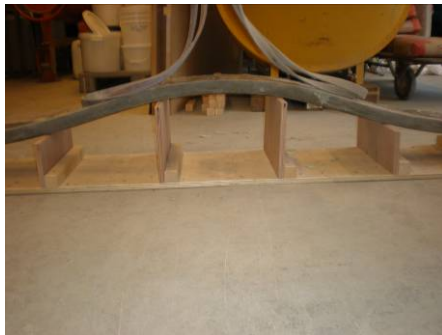
Figure 8-39: Demoulded element at the supports
