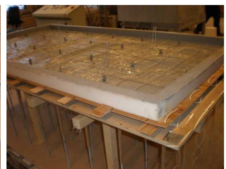
Figure 10-26: Mould at horizontal position
