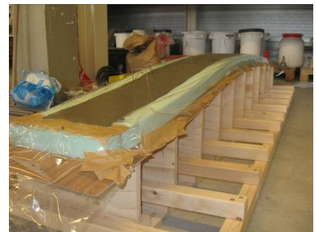
Figure 8-6: Just deformed concrete
