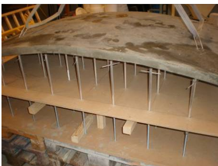
Figure 10-18: Unmolded element placed on the supports
