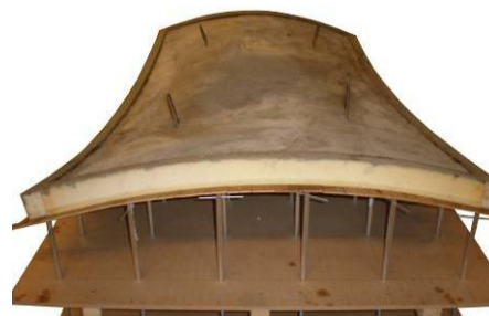
Figure 16: Double curved element at the flexible formwork
