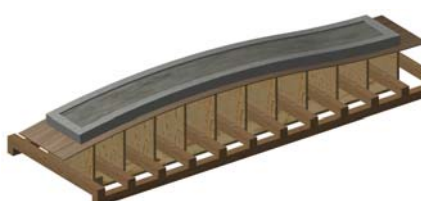
Figure 10: Deformed mould and concrete
