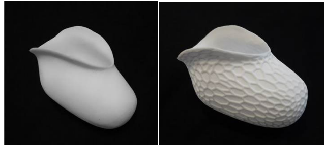
Figure 1. Transradial anatomically contouring socket by Strömshed (2017). a) Smooth design. b) Lattice pattern design.
