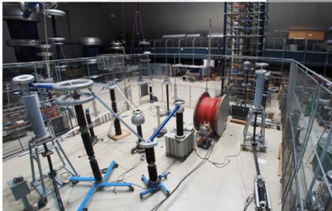
Fig. 15. Superimposed impulse test circuit used for acquiring the data sets 1 and 2. More details can be found in [16].
