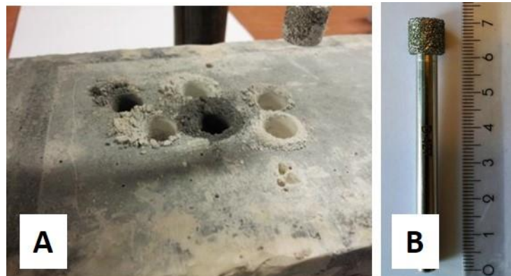
Figure 6.2 (a) An example of drilled holes for determination of chloride concentration profiles at the exposed zone of specimens; (b) drill bit
