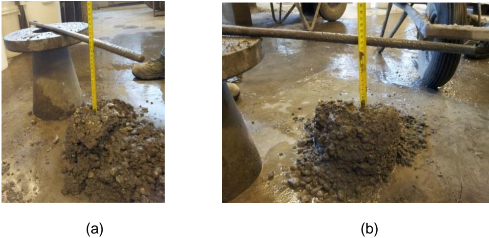
Figure 5.2 Slump test of (a) normal strength concrete and (b) bacterial concrete
