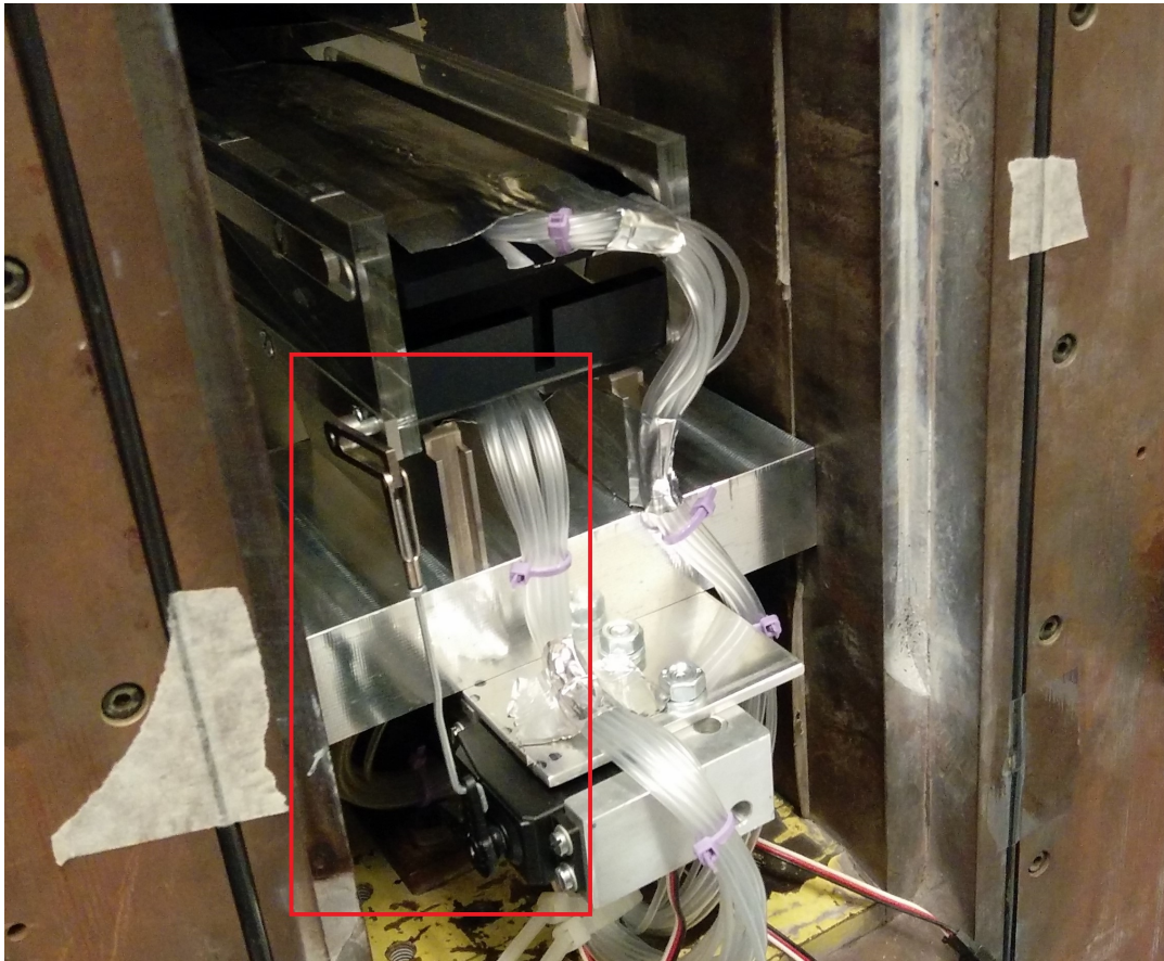
Figure 3.8: Picture of the actuation system that drives the mass flow control valve at the back of the intake
