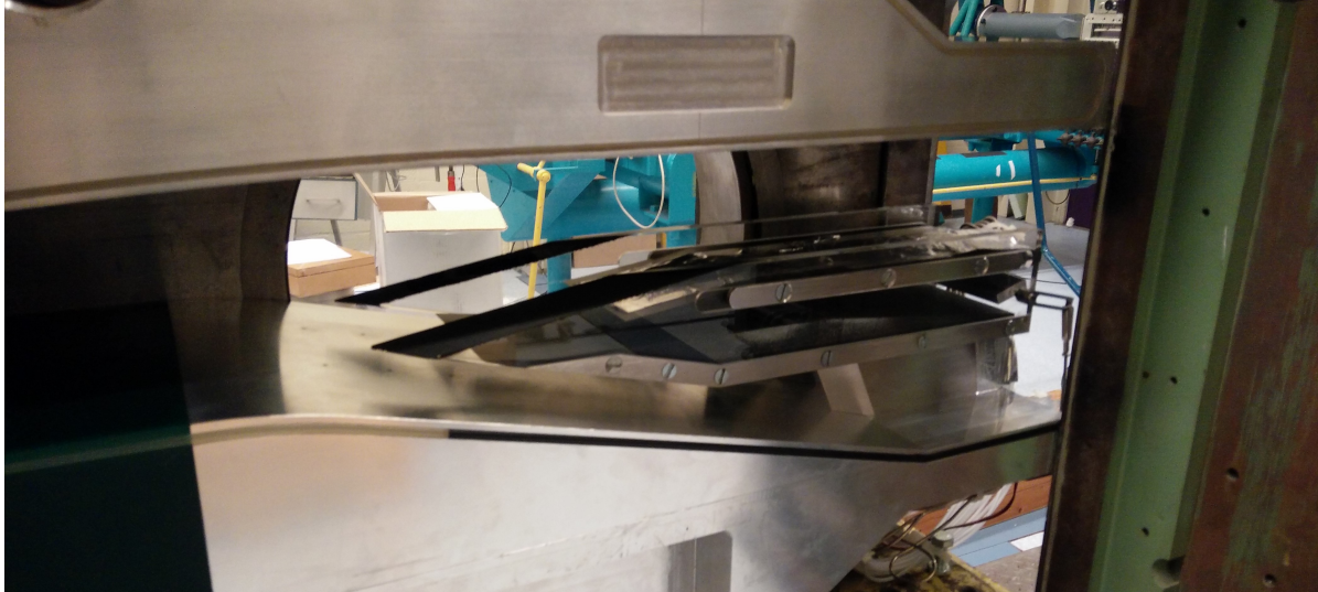
Figure 4.2: The submerged supersonic intake model in the double shock configuration in the test section of the ST-15.
