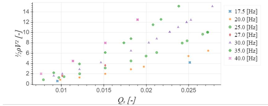
Figure 4.14: flow velocity squared vs specific capacity for HRMD3B at different shaft speeds
