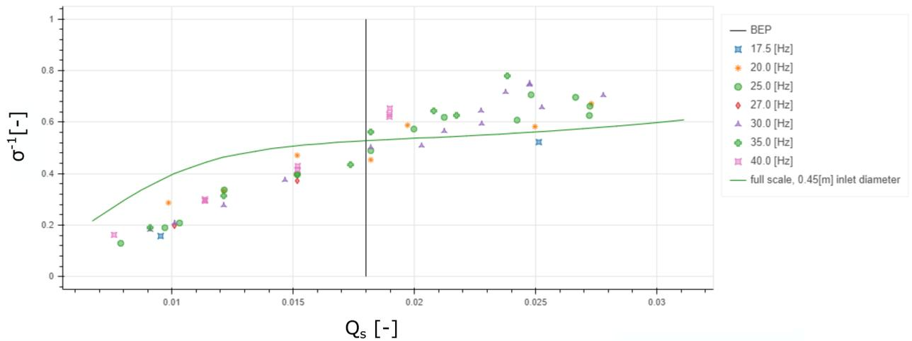
Figure 4.18:  $\sigma^{-1}$  for 0.1 m inlet diameter at different shaft speeds and 0.45 m inlet diameter
