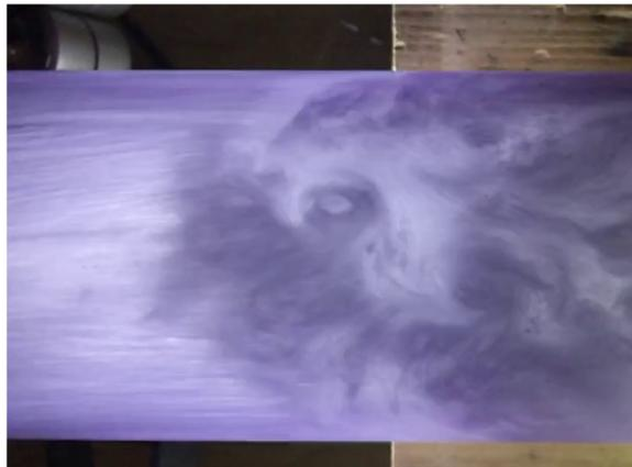
Figure 3.30: cavitating valve
