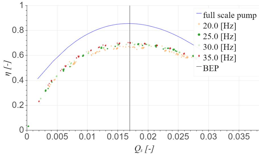
Figure 4.17:  $\eta$  vs  $h_s$  for the 0.1 [m] HRMD3B pump at different shaft speeds and the full scale pump (0.45 [m])
