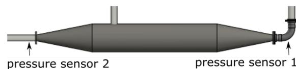
Figure 3.7: sensors for pressure differential over water tank
