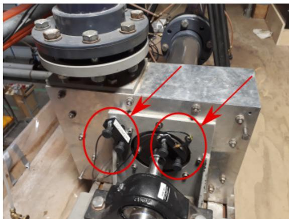
Figure 3.22: acoustic sensor locations
