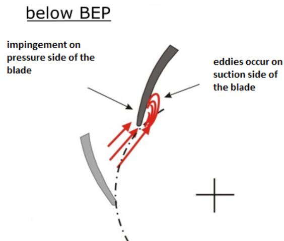
Figure 1.7: Flow profile in centrifugal pump below BEP
