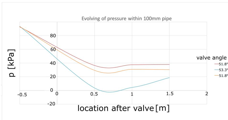
Figure 3.32: Pressure development after butterfly valve.
