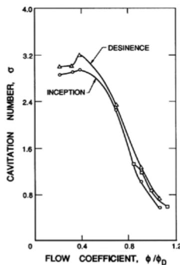
Figure 2.7: Cavitation hysteresis (Brennen 1994)
