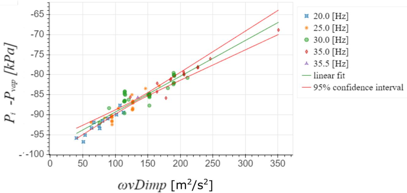
Figure 4.26: inlet pressure vs  $\omega \vec{v} D_{imp}$
