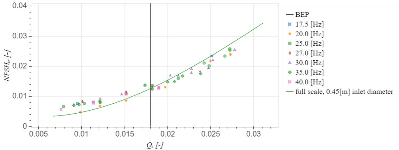
Figure 4.20: Specific  $NPSH_r$  for 0.1 m inlet diameter at different shaft speeds and 0.45 m inlet diameter
