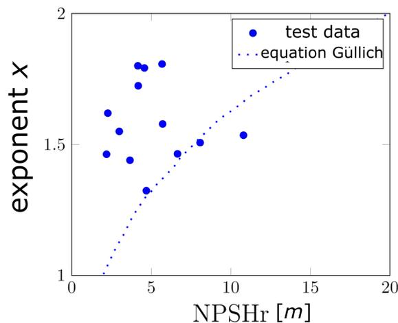
Figure 2.12: Exponent according to equation 2.25, based on manufacturer data. From Güllich (2010)
