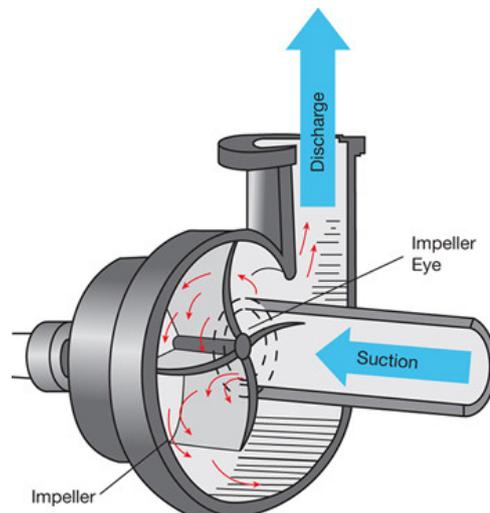
Figure 1.1: flow through centrifugal pump, source: <https://www.pumpfundamentals.com>
