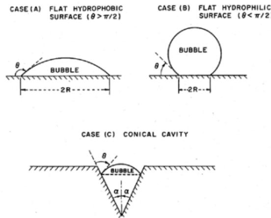
Figure 2.10: example of heterogenous nucleation after Brennen (1995)
