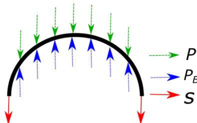
Figure 2.9: schematical presentation of forces acting on half of a bubble
