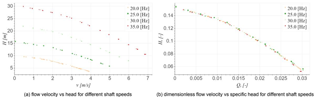
Figure 4.2: head vs flow velocity and specific head vs specific capacity of a HRMD3B impeller. Measurements performed in this research.
