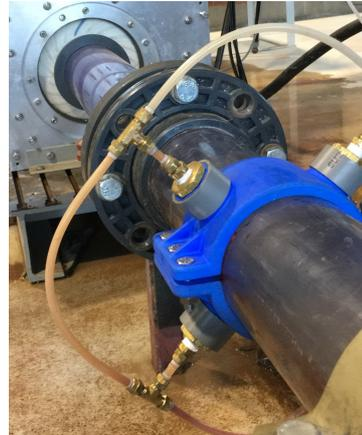
(b) 3d printed pressure sensor housing, courtesy J. Hoebe
