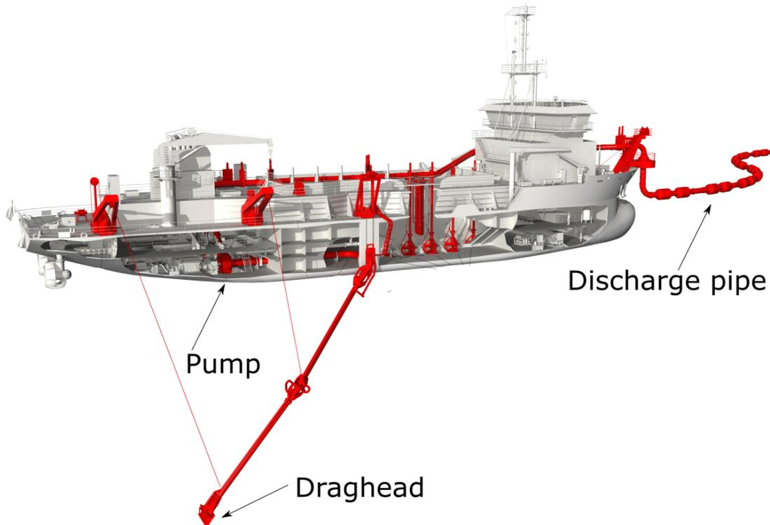
Figure 1: Trailing Suction Hopper Dredge
