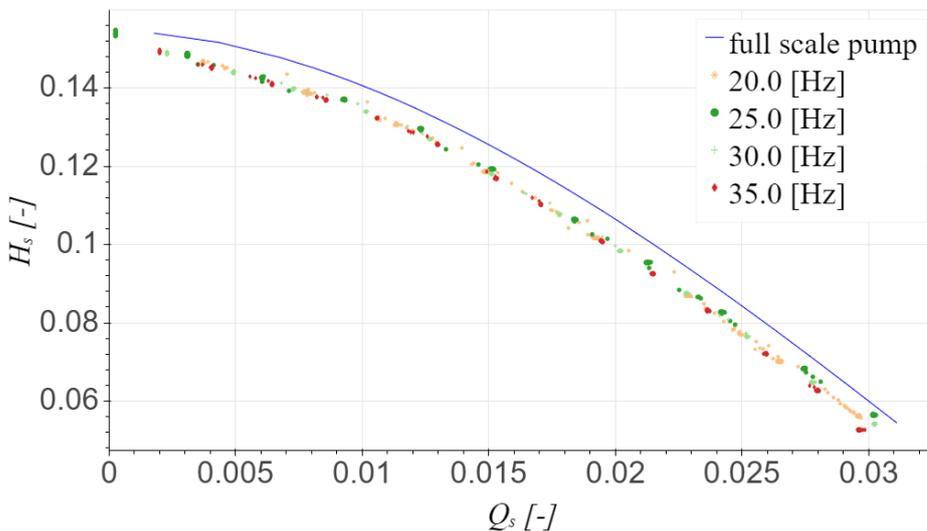
Figure 4.16:  $Q_s$  vs  $h_s$  for the 0.1 [m] HRMD3B pump at different shaft speeds and the full scale pump (0.45 [m])
