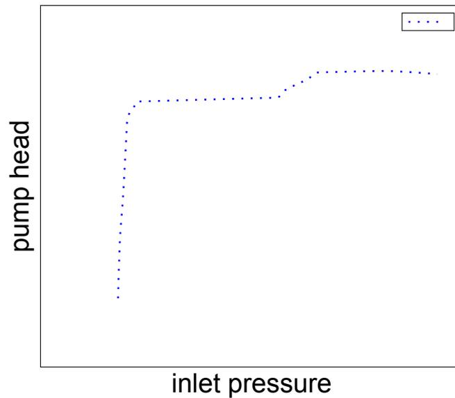
Figure 2.17: Typical alternating vane cavitation
