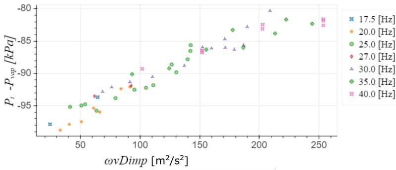
Figure 4.15: Inlet pressure minus vapour pressure vs flow velocity\*speed\*diameter for HRMD3B at different shaft speeds
