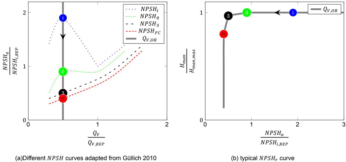
Figure 2.5: typical  $NPSH_r$  measurements, for a constant speed
