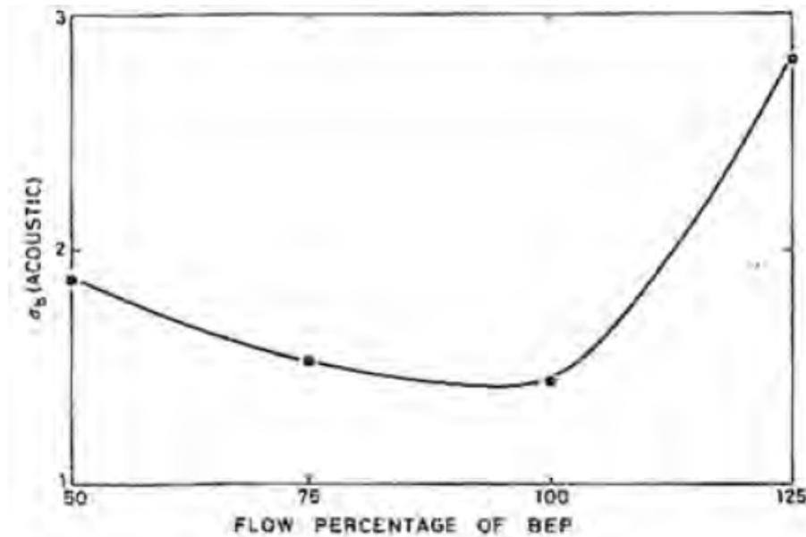
Figure 2.19: acoustic cavitation number vs flow Schiavello and Visser (2009)
