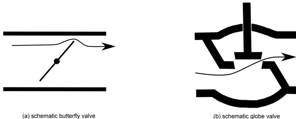
Figure 3.33: schematic presentation valves
