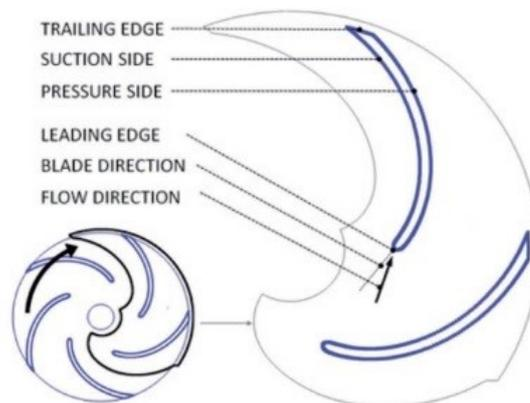
Figure 1.5: identifying pressure side, suction side, leading and trailing (Went 2018)
