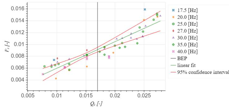
Figure 4.22: linear of specific inlet pressure and specific capacity at  $NPSH_r$  for different shaft speeds
