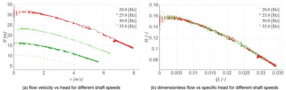
Figure 4.4: head vs flow velocity and specific head vs specific capacity of a HRMD4B-curve impeller. Measurements performed in this research.
