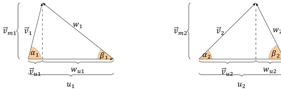
Figure 1.4: Velocity triangles; inlet (left), exit (right)
