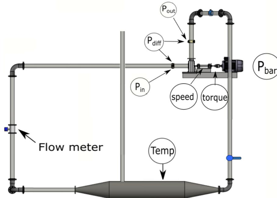
Figure 4.1: test setup, with sensors
