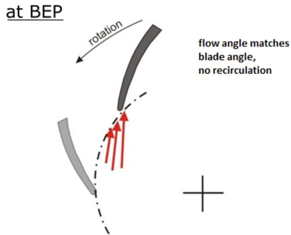
Figure 1.6: Flow profile in centrifugal pump at BEP
