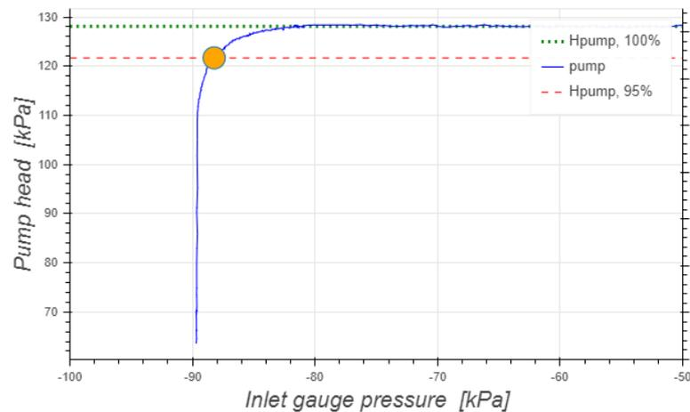
Figure 3.21: HRMD4b-curve  $NPSH_r$  measurement, shaft speed 25[Hz], flow velocity 3 [ $\frac{m}{s}$ ]
