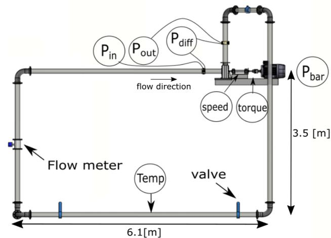
Figure 3.3: combining those sensors and making a loop for the pump to operate
