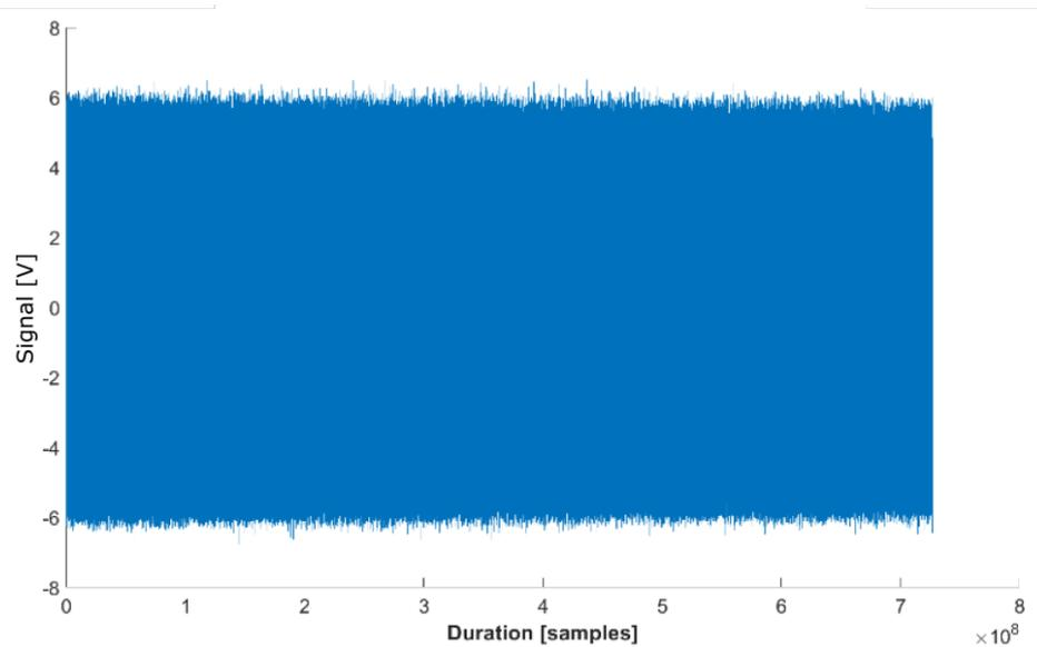
Figure 3.23: Saturated acoustic emission sensor, sample frequency  $10^{-6}$ Hz
