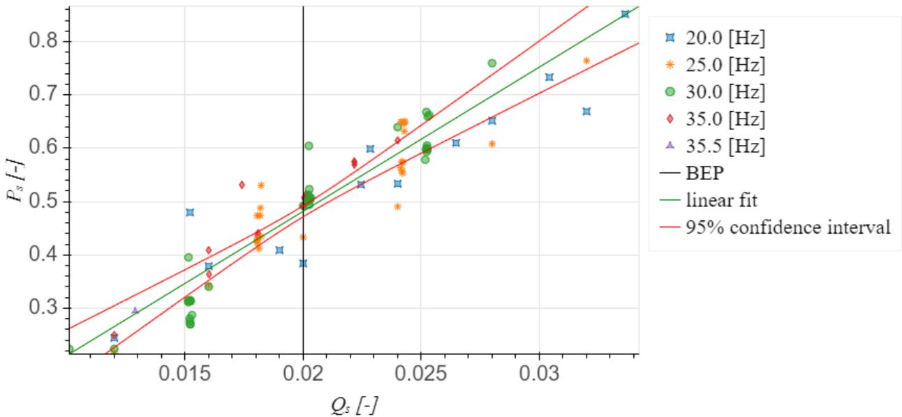
Figure 4.25: Specific pressure vs specific capacity for HRMD4B-curve
