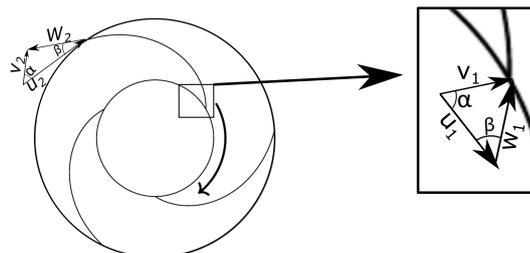
Figure 1.3: Velocity triangles in 2d impeller representation
