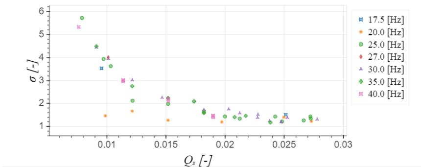
Figure 4.12: Cavitation number vs specific capacity for HRMD3B at different shaft speeds
