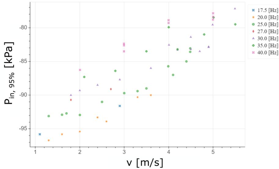
Figure 4.9: Absolute inlet pressure vs flow velocity for HRMD3B at different shaft speeds
