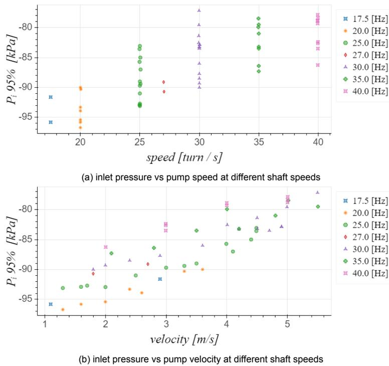
Figure 4.21: Inlet pressure vs speed and velocity
