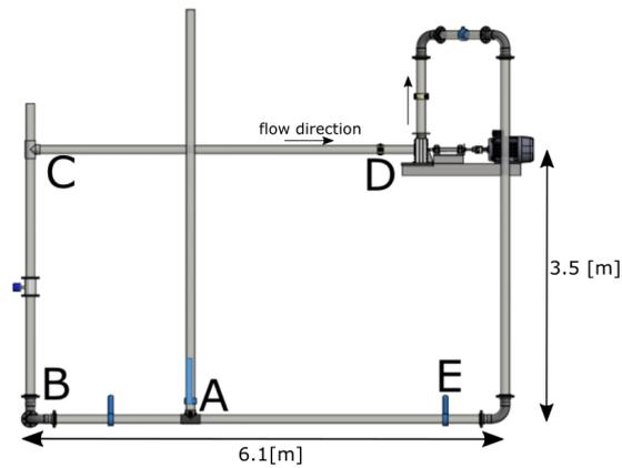
Figure 3.1: First pump setup, courtesy J. Hoebe
