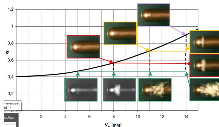
Figure 2.13: cavitation on a hemispherical object( Keller 2001)
