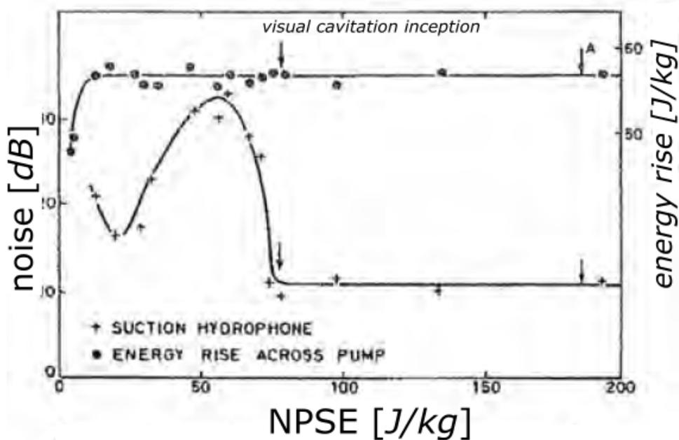
Figure 2.18: cavitation noise as a function on inlet pressure Schiavello and Visser (2009)
