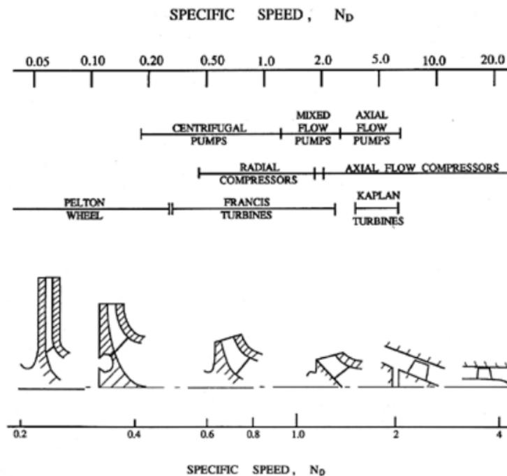
Figure 1.2: Pump design specific speed after Brennen (1994)
