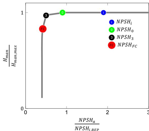
Figure 3.20: qualitative  $NPSH_r$  measurement
