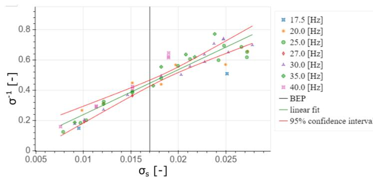
Figure 4.23: fit and confidence interval of  $\sigma^{-1}$
