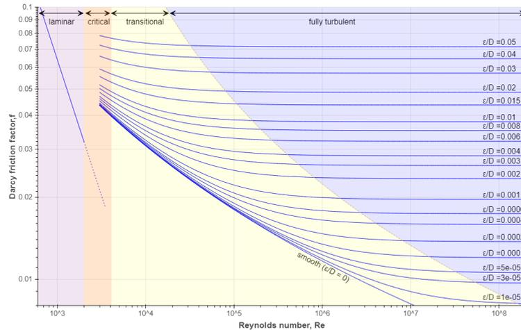
Figure 2.11: Moody diagram, adapted from D. G. Hyams
