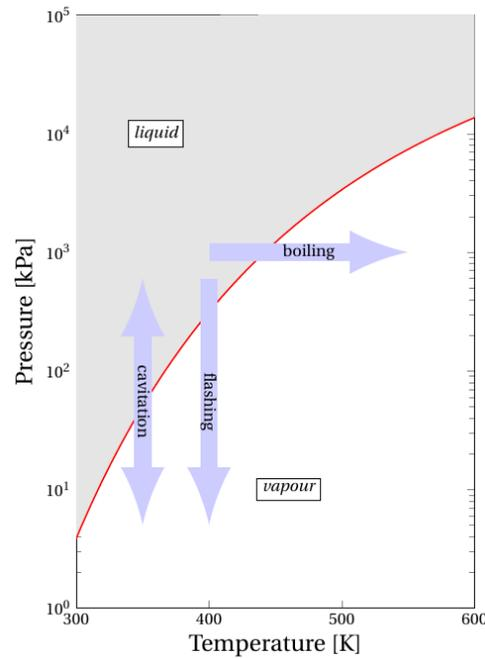
Figure 2.2: cavitation, flashing and boiling
