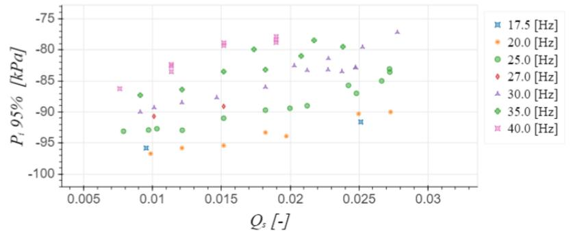
Figure 4.10: Absolute inlet pressure vs specific capacity for HRMD3B at different shaft speeds
