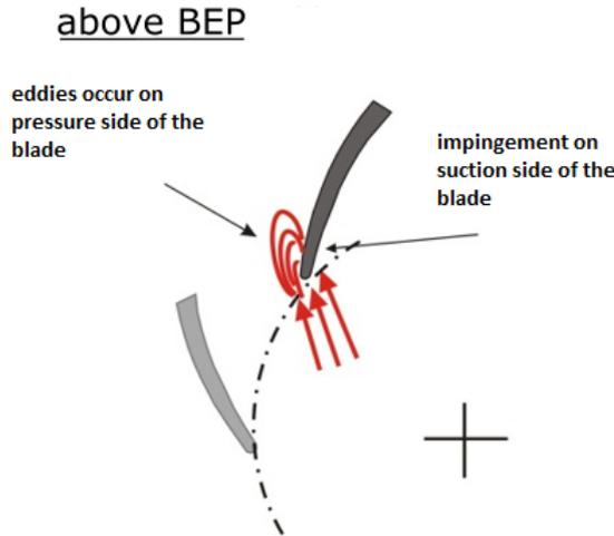
Figure 1.8: Flow profile in centrifugal pump above BEP
