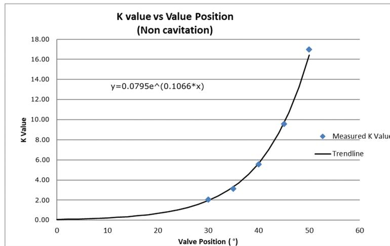
Figure 3.31: Obstacle factor in a non cavitating valve
