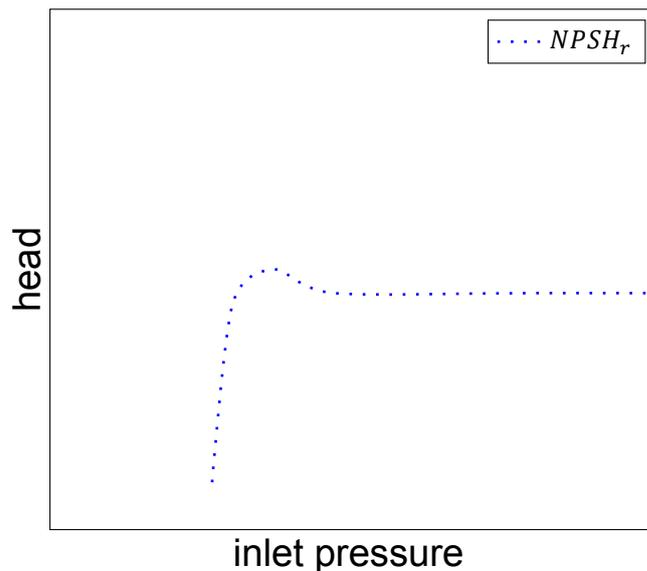
Figure 2.15:  $NPSH_r$  with pre-liminary increased efficiency
