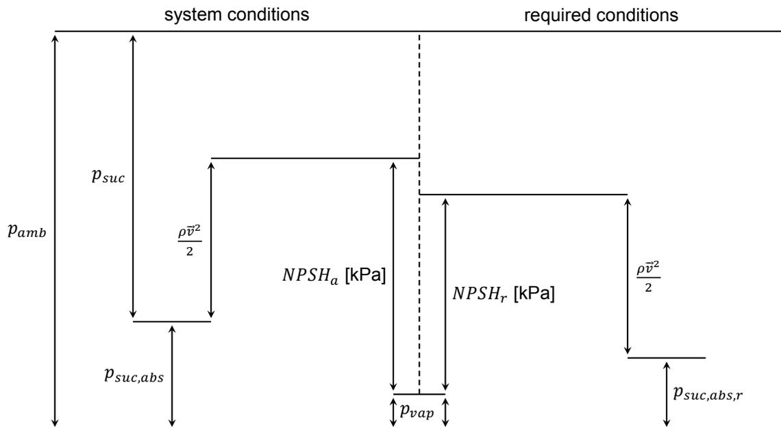
Figure 1.10: Schematic view of parameters relating to inlet pressure, after Berg (2013)
