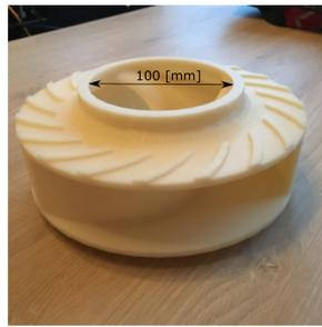
Figure 3.11: 3D printed nylon impeller
