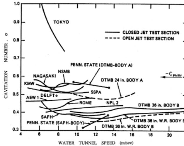
Figure 2.8: Cavitation inception tests: Brennen (1995)
