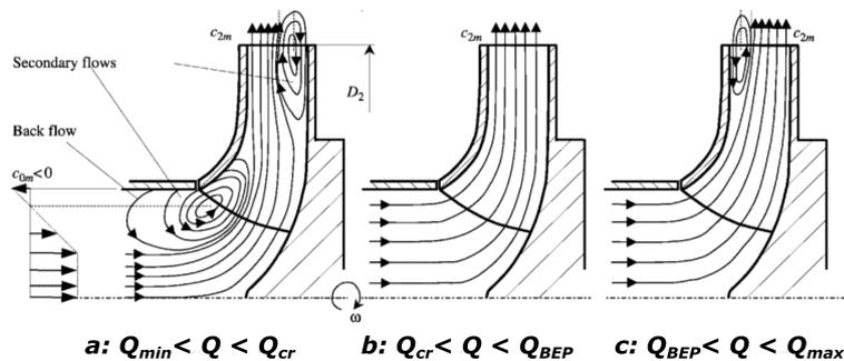
Figure 1.9: secondary flow in impeller, causing pre-rotation (Predin and Biluš 2003)
