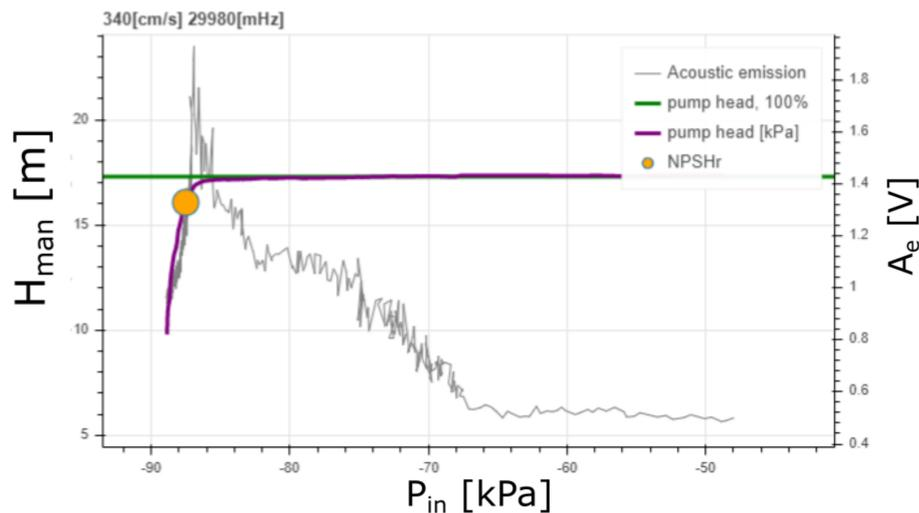
Figure 3.26: AE measurement without local maximum
