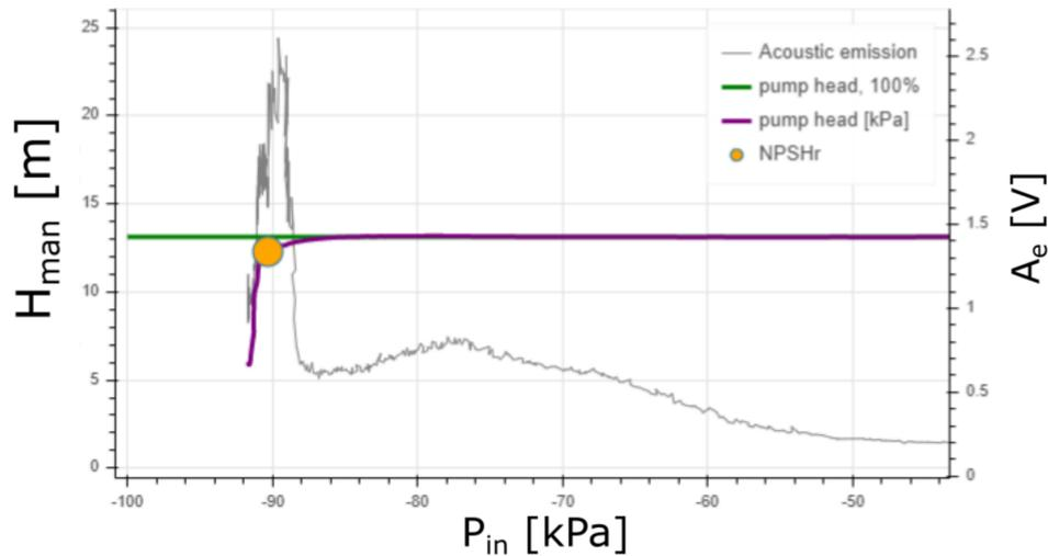
Figure 3.25: Acoustic emission measurement with local maximum
