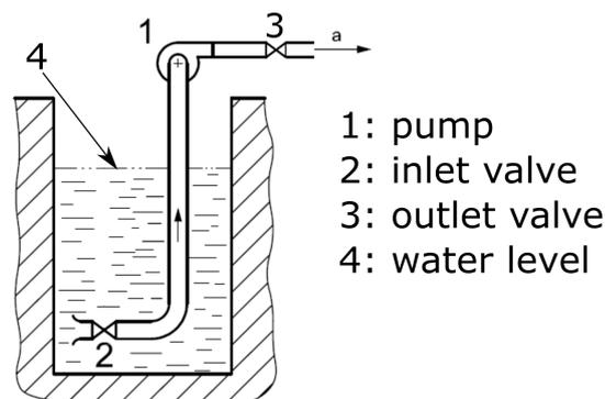
Figure 3.19: open sump setup, adapted from ISO (2012)
