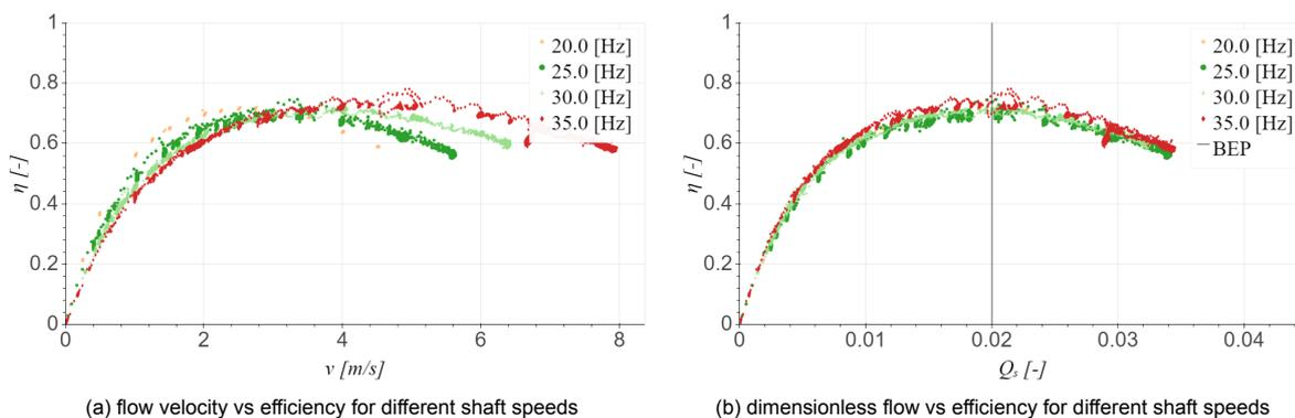
Figure 4.5: efficiency vs flow velocity and specific capacity of a HRMD4B-curve impeller. Measurements performed in this research.
