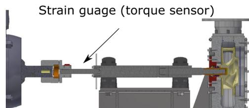
Figure 3.9: location torque sensor
