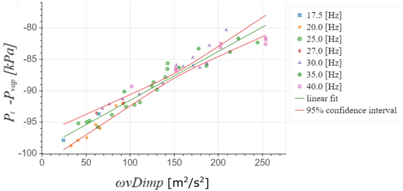
Figure 4.24: inlet pressure vs  $\omega \bar{v} D_{imp}$
