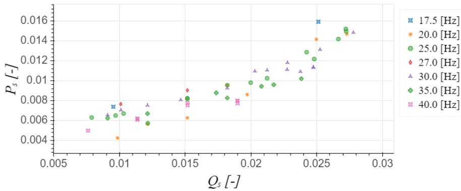
Figure 4.11: Specific inlet pressure vs specific capacity for HRMD3B at different shaft speeds
