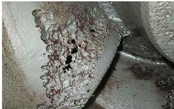
Figure 2.4: Cavitation damage, source: <https://www.empoweringpumps.com>
