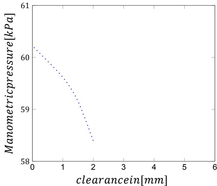
Figure 3.15: relation between clearance and manometric pressureP
