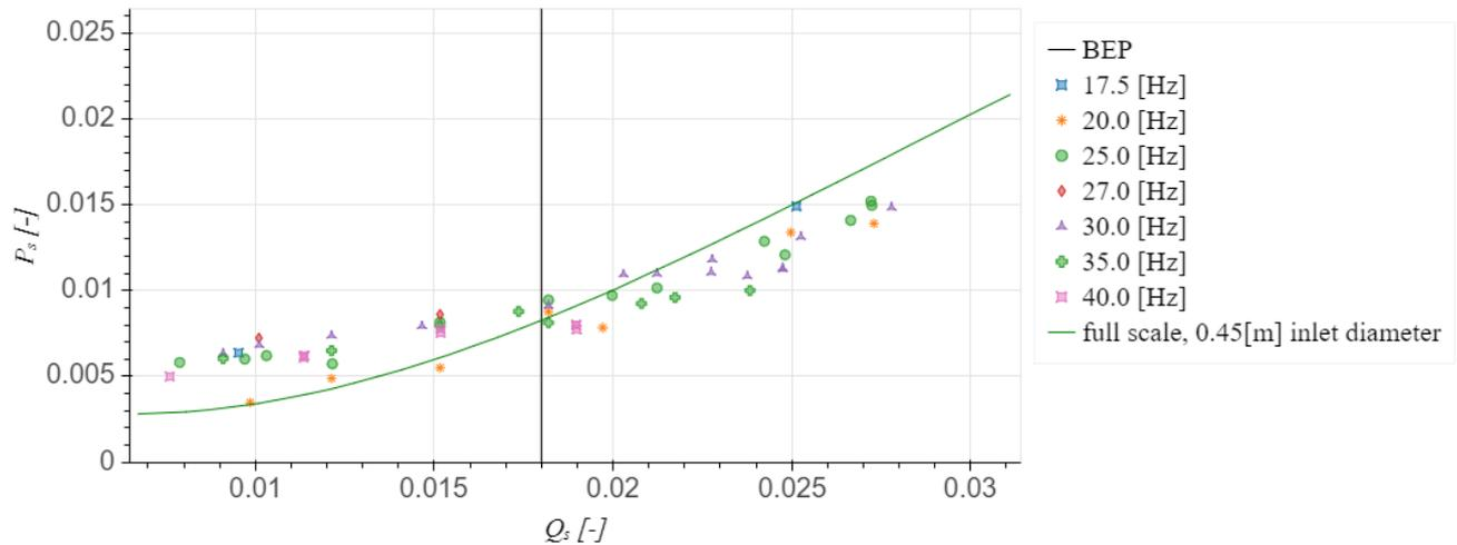
Figure 4.19: Specific inlet pressure for 0.1 m inlet diameter at different shaft speeds and 0.45 m inlet diameter
