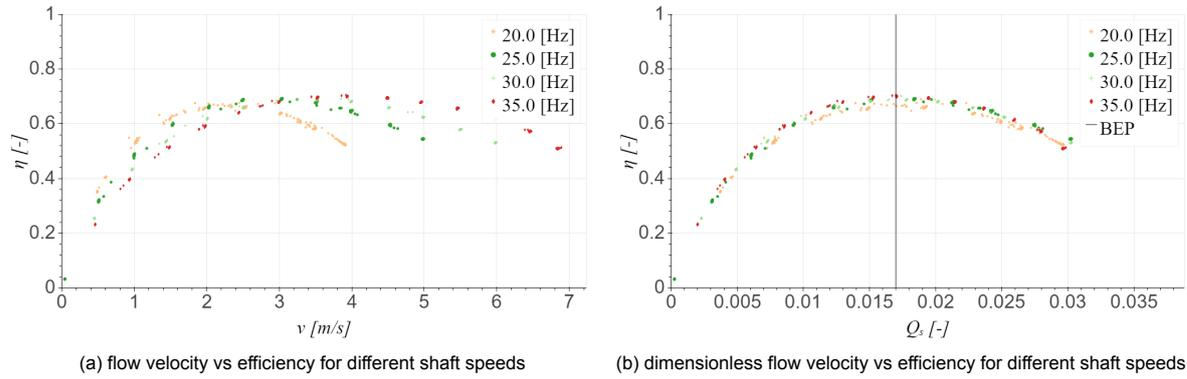
Figure 4.3: efficiency vs flow velocity and specific capacity of a HRMD3B impeller. Measurements performed in this research.
