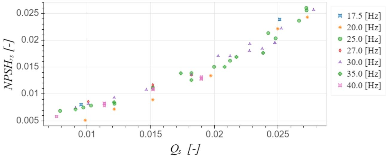
Figure 4.8: Specific NPSHr for  $D=0.45$  m and 0.1 m inlet diameter for different shaft speeds
