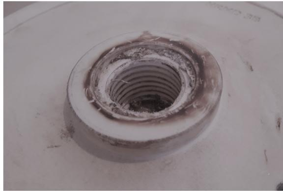
Figure 3.13: worn out impeller connection
