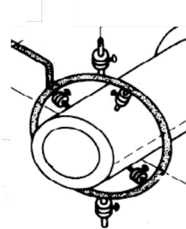
(a) point pressure sensor connection, from ISO-5198 (1998)
