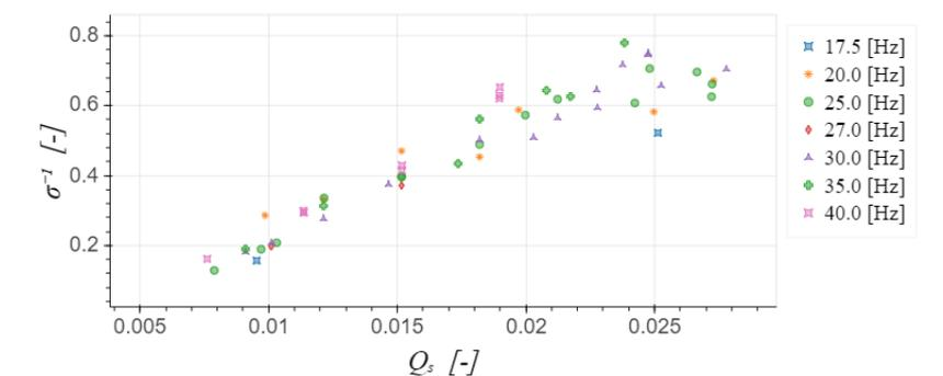
Figure 4.13: reciprocal of cavitation number vs specific capacity for HRMD3B at different shaft speeds
