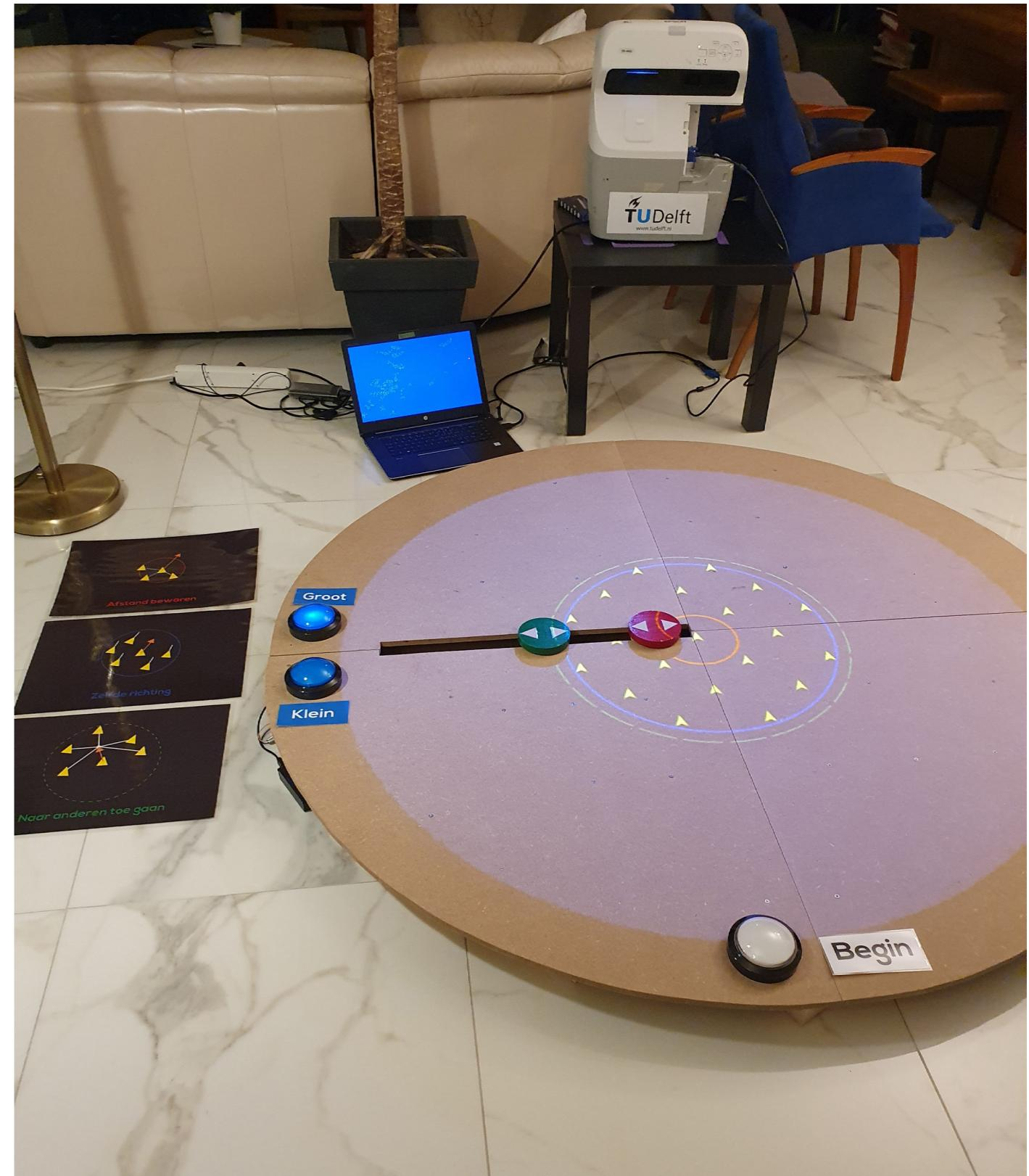
Figure 76: Prototype that is used for the validation in Naturalis. The two disks to move the sliding mechanism are painted in the colour of the corresponding circle, to let the user know which disk corresponds to which circle. Arrows are added on top to give users the use-cue that they are movable. The buttons are annotated with the words 'small' and 'large' for orientation and 'restart' for the restart button.
