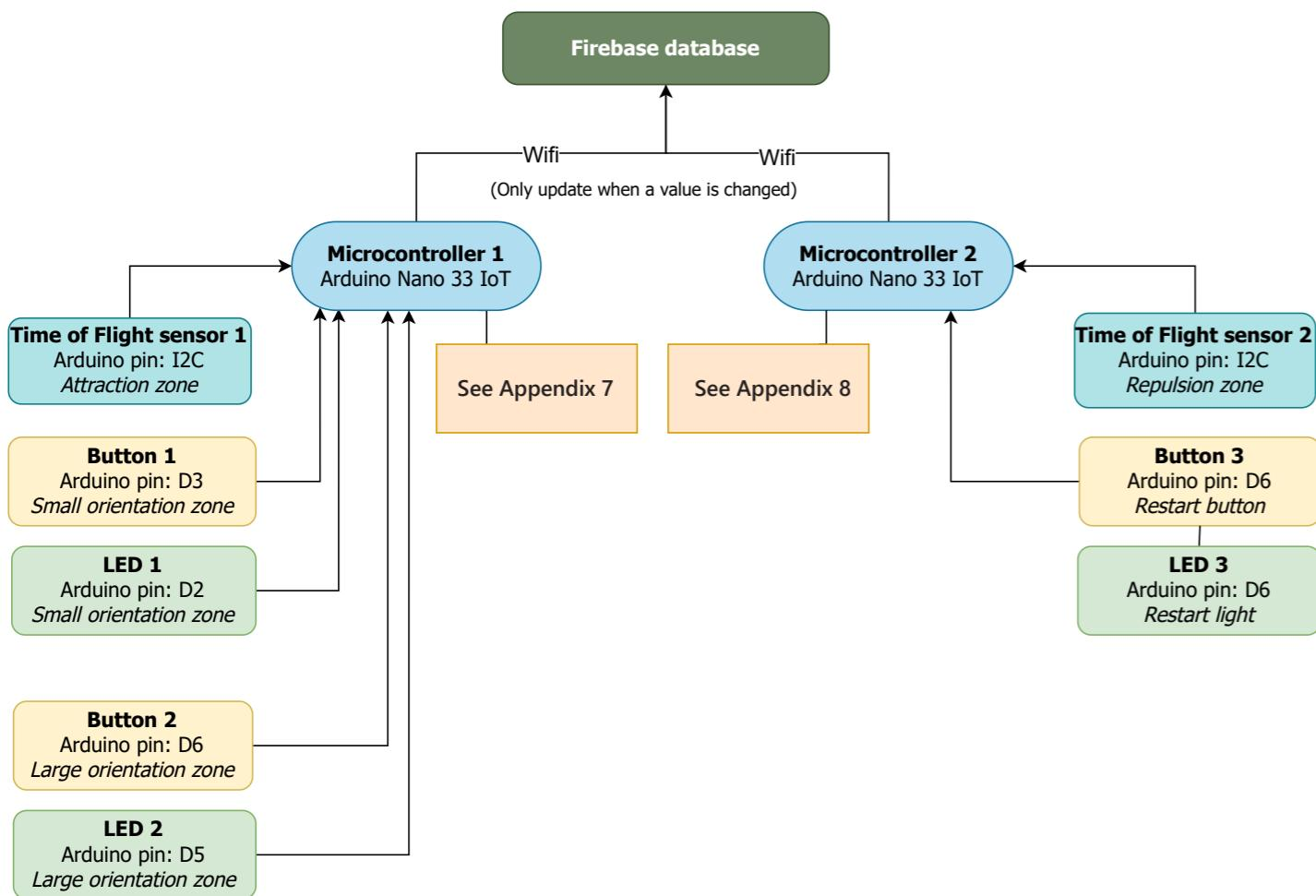
Figure 69: System diagram of both Arduino boards.
