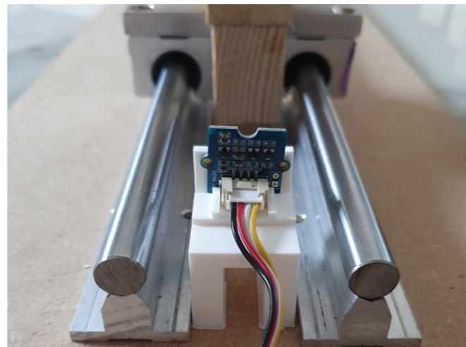
Figure 74: Chosen 3D print for time of flight sensor holder
