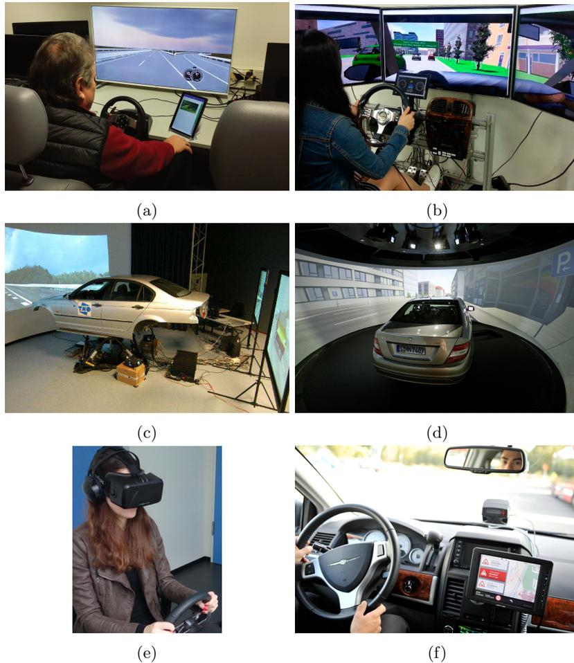
Figure 2. (a) shows a NIVR (Holländer & Pfleging, 2018), (b) shows a SIVR<180 (Eom & Lee, 2015), (c) shows a SIVR>180, (d & e) show a TIVR (Hock et al, 2016; "New driving simulator taken into operation in Sindelfingen: Investment in cutting-edge technologies," 2010) and (f) shows a real driving experiment (Farah & Koutsopoulos, 2012).
