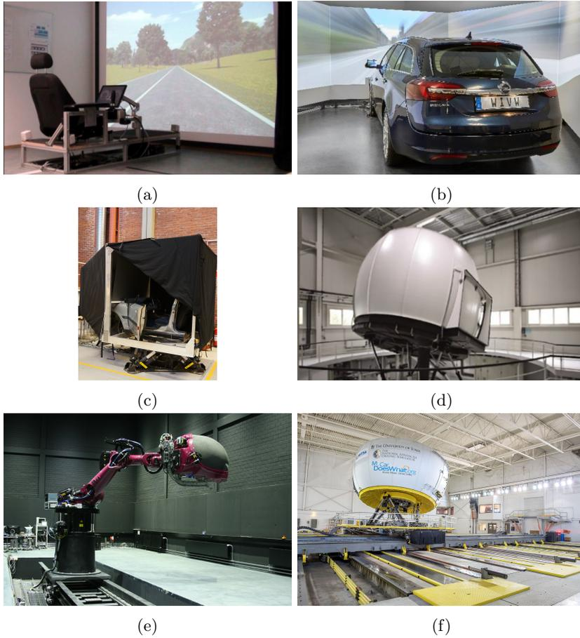
Figure 3. (a) & (b) show a FB configuration (Befelein et al., 2018; Damböck et al., 2011), (c) & (d) show a 6 DOF MB configuration (Forster et al., 2019; Nilsson et al., 2013), (e) shows a 8 DOF MB configuration (Sadeghian Borojeni et al., 2018) and (f) shows a 13 DOF MB configuration (National Advanced Driving Simulator Overview, 2010).
