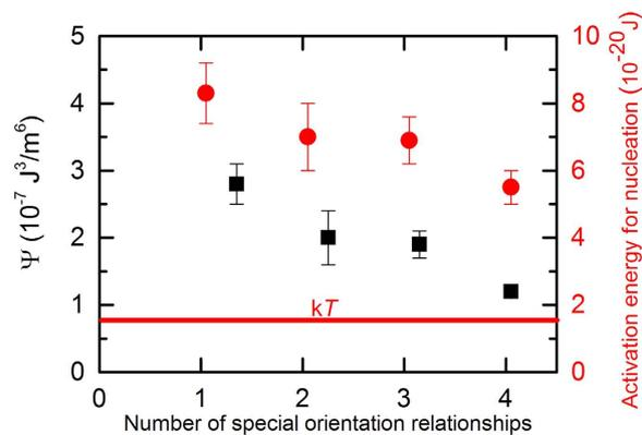
**Figure 4. Critical nucleus parameters.** The fitted values for the  $\Psi$ -parameter (squares) and the activation energy for nucleation (circles) as a function of the number of special OR's between austenite and ferrite grains. Note: the error bar of the value for the  $\Psi$ -parameter for four special OR's is equal to the symbol size.
