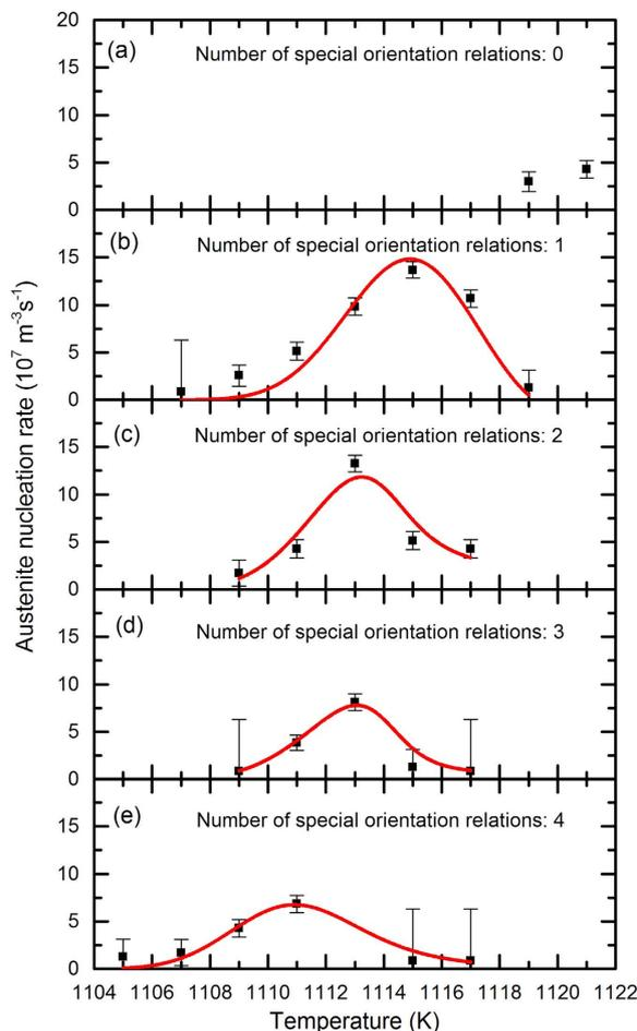
**Figure 3. The austenite nucleation rate as a function of temperature.** The number of special ORs is (a) 0, (b) 1, (c) 2, (d) 3, and (e) 4. The solid lines indicate fits of the classical nucleation theory to the experimental data (squares).
