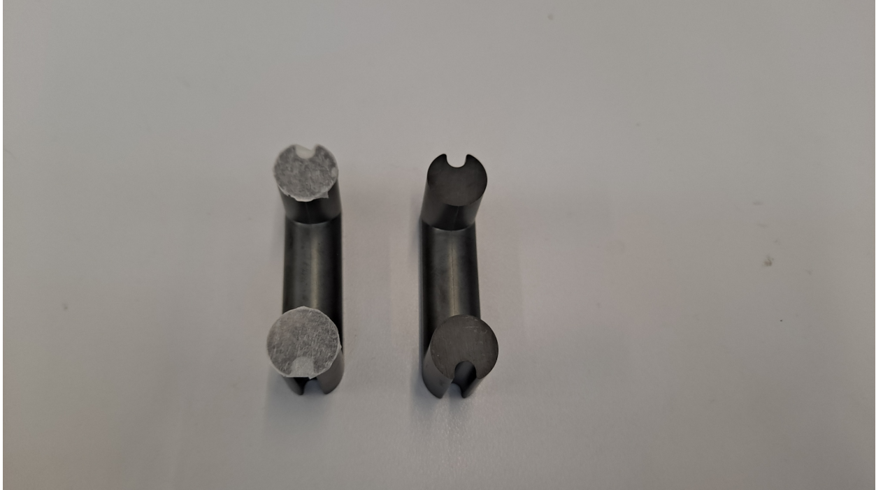
Figure D.5: The ferrite core with added tape "air gap" to reduce inductance.
