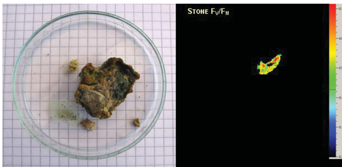
Fig. 9. The Stone sample. The fluorescence measurements reveal the photochemically active region.
