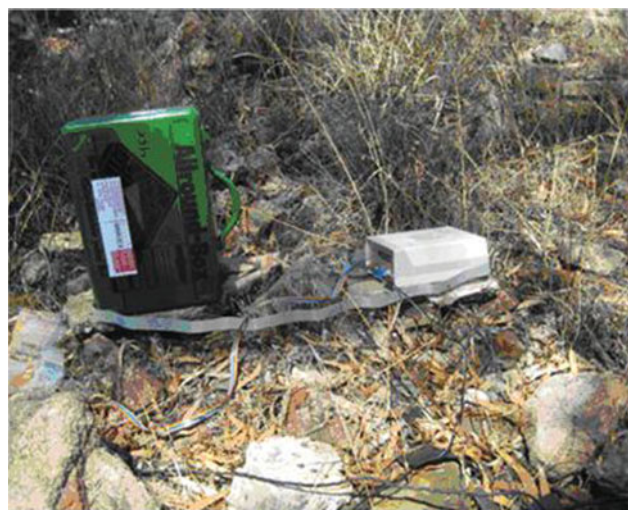
Fig. 6. Mössbauer spectrometer MIMOS II in measuring position. The sensor head can be placed in any direction depending on the sample to be analysed.
