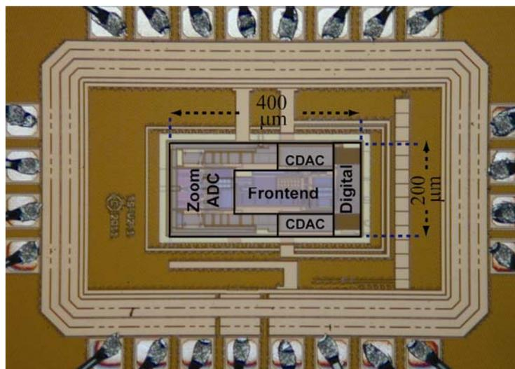
**Fig. 10** Chip micrograph of the sensor.
