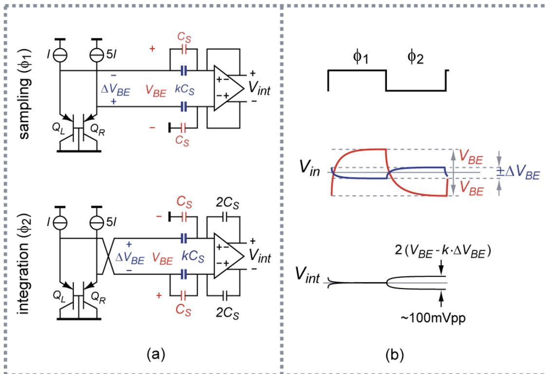
**Fig. 6** (a) Proposed integration scheme during sampling ( $\phi_1$ ) and integration ( $\phi_2$ ) phases. (b) Waveforms of a full SAR/ $\Delta\Sigma$  cycle.  $V_{in}$ : zoom ADC's input voltage,  $V_{int}$ : integrator's output voltage. Parameter  $k$  is set by the SAR logic in the coarse conversion, while  $k = n-1$  or  $n+1$  when  $bs = 0$  or  $1$  in the fine conversion step.
