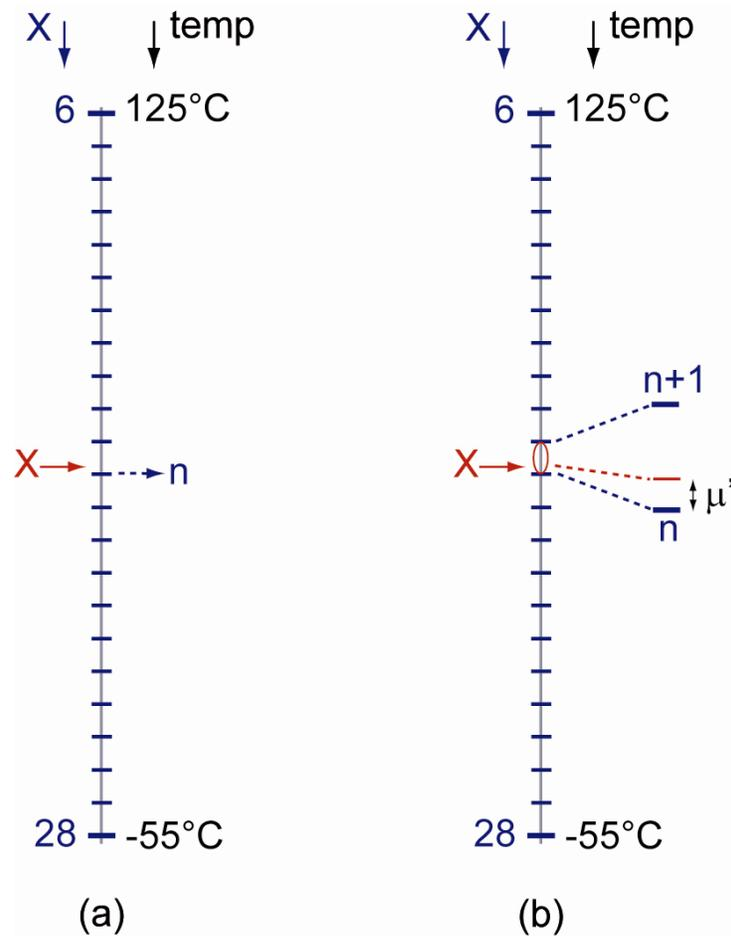
**Fig. 3** Temperature dependence of  $X = n + \mu'$  from  $-55^\circ\text{C}$  to  $125^\circ\text{C}$ . The integer  $n$  ranges between 6 and 28 (a) while the fraction  $\mu'$  ranges between 0 and 1 (b).
