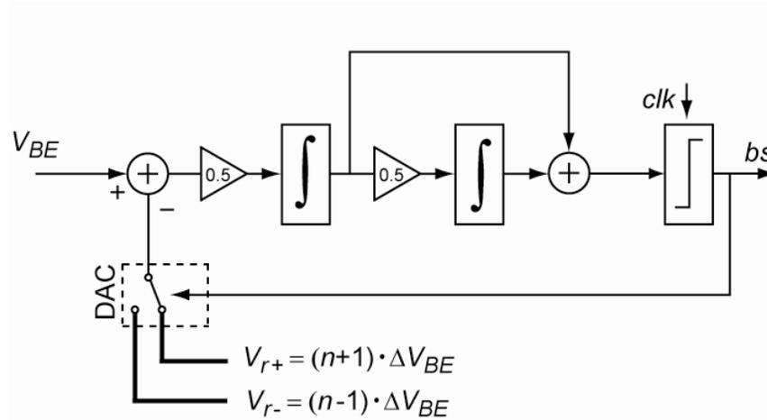
**Fig. 5** Block diagram of the proposed 2<sup>nd</sup>-order zoom ADC during the fine conversion.
