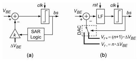
Fig. 4 Block diagram of the zoom ADC during the coarse (a) and fine (b) conversions.
