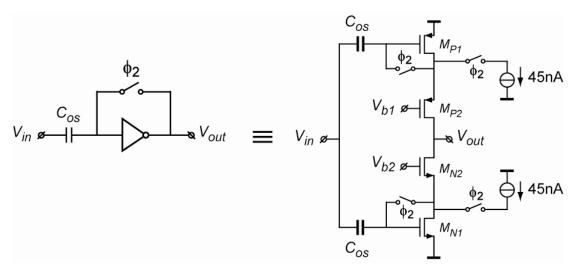
**Fig.8** Circuit diagram of the proposed inverter-based OTA.
