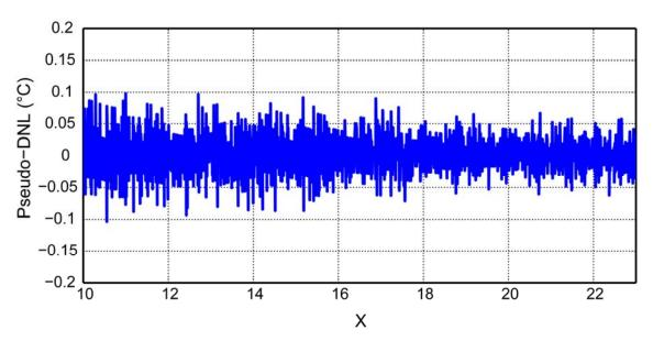
**Fig. 15** Measured Pseudo-DNL versus *X*. The sensor's conversion time is 5.3msec.
