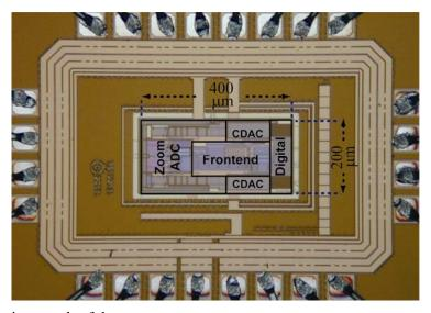
Fig. 10 Chip micrograph of the sensor.
