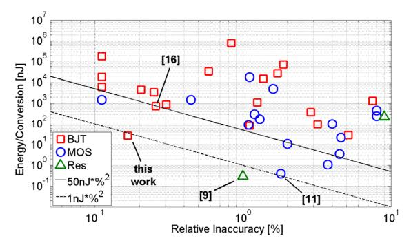
**Fig. 17** Energy per conversion versus relative inaccuracy for different smart temperature sensors using different sensing principles [12].
