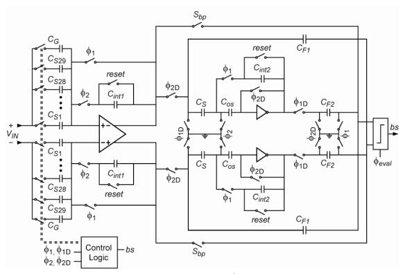
Fig. 7 Simplified circuit diagram of the proposed 2<sup>nd</sup>-order zoom ADC.
