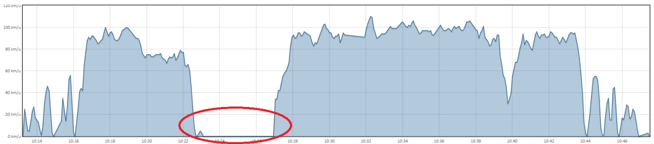
Figure A.20 – Speed profile of a participant's test drive in which the bridge opening on the A20 is clearly visible
