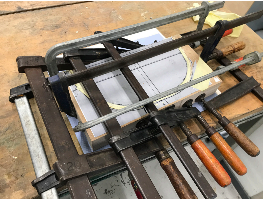
Figure 6: The airplane triplex inbetween the mould
