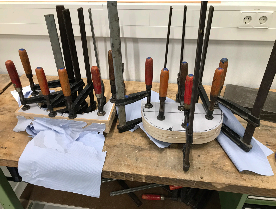
Figure 5: the lasercut mould parts glued together
