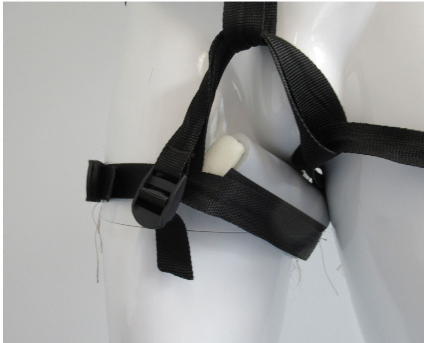
Figure 70: Concept with extra padding. Note that in this picture only one side has the extra padding as the other pad did not fit on the mannequin as well.
