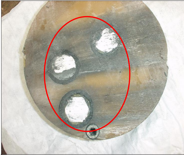
Figure 2.6: Conductor displacement inside a resin insulated joint [5].
