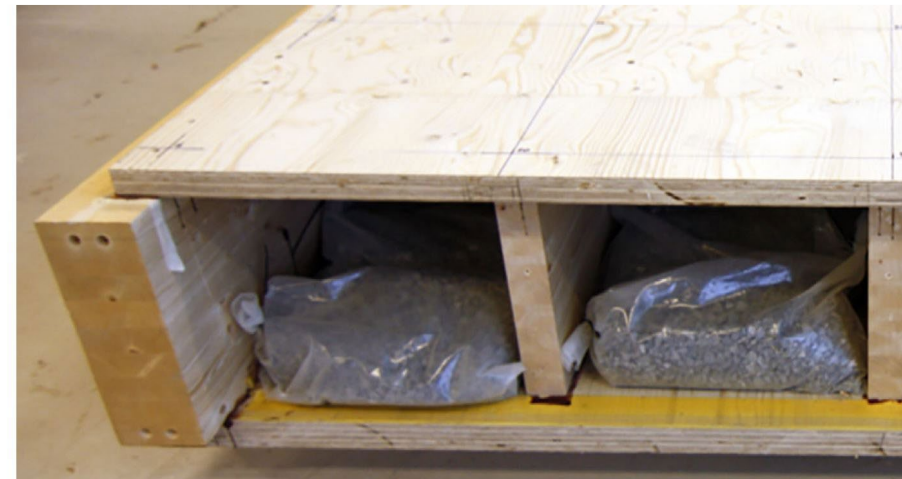
Fig. 6. Element cavity with the gravel bags.
