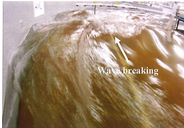
Figure 4-15. Wave quality for model 11-12 B = 275\text{mm} with d^* = 0.2 in h_0 = 250\text{mm} and \kappa \approx 0 at Fr_{h_0} = 0.99 at with \alpha = 14^\circ rear view at water level. The arrow indicates local wave breaking.
