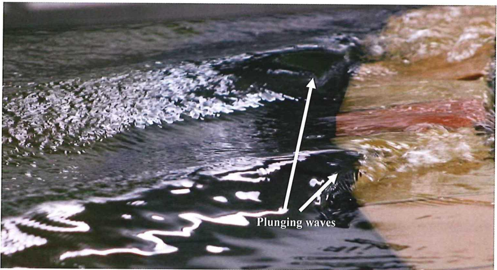
Figure 2-6. Plunging waves (first and second waves) generated by condition 56 model 12-02 with \xi = 1 , d^* = 0.2 in h_0 = 250\text{mm} at Fr_{h_0} = 0.95 and s = 17^\circ and y_{beach}^* = 1.9 .
