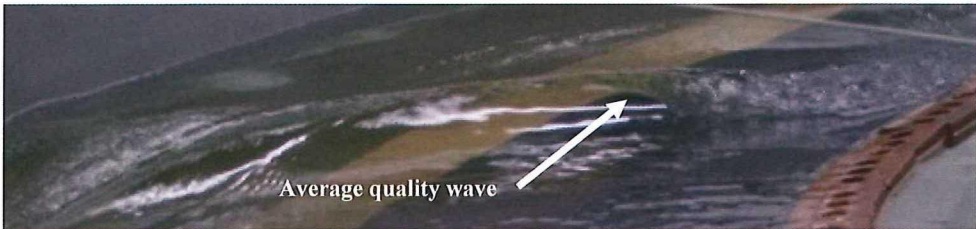
Figure 3-10. Example of an average quality wave for condition 48 model 12-02 with d^* = 0.2 in h_0 = 250\text{mm} at Fr_{h_0} = 0.95 , \kappa = 0.07 , s = 17^\circ and y_{beach}^* = 1.4 .
