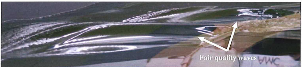
Figure 3-9. Example of fair quality waves for condition 57 model 12-02 with d^* = 0.2 in h_0 = 250\text{mm} at Fr_{h_0} = 0.95 , \kappa = 0.06 , s = 17^\circ , and y_{beach}^* = 1.9 .
