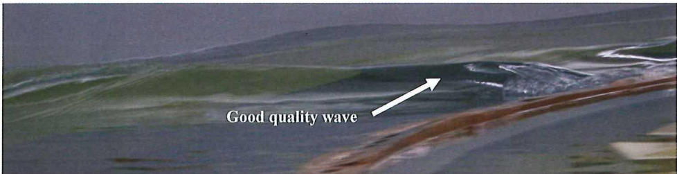
Figure 3-11. Example of a good quality wave for condition 55 model 12-02 with d^* = 0.2 in h_0 = 250\text{mm} at Fr_{h_0} = 0.95 , \kappa = 0.07 , s = 17^\circ and y_{beach}^* = 1.4 .
