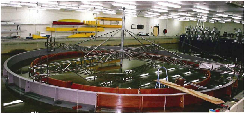
Figure A-10. Circular track scale model with wall at y = 888\text{mm} .
