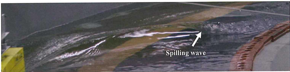
Figure 2-5. Spilling wave generated by condition 48 run 402 model 12-02 with \xi = 0.4 , d^* = 0.2 in h_0 = 250\text{mm} at Fr_{h_0} = 0.95 and s = 9^\circ and y_{beach}^* = 1.4 . The pressure source was travelling towards the camera.
