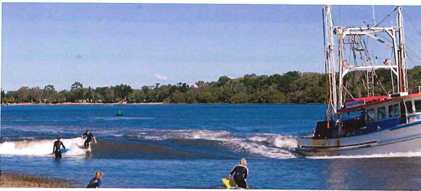
Figure 2-21. Trials using a fishing vessel on a river to generate surfable waves (reproduced with permission of Liquid Time Pty Ltd).
