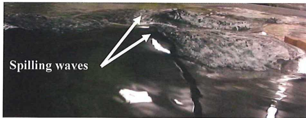
Figure 5-8. Spilling waves generated by condition 63 model 12-03 R_0^* = 6 and \kappa = 0.07 with d^* = 0.2 in h_0 = 500\text{mm} water depth, y_{beach}^* = 1.9 at Fr_{h0} = 0.95 .
