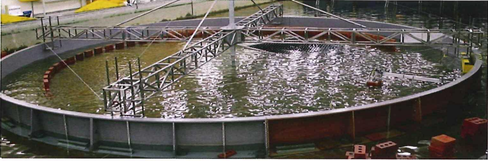
Figure A-11. Circular track scale model with no sloping beach or wall.
