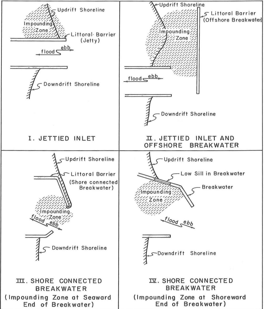
FIGURE I. TYPES OF LITTORAL BARRIERS WHERE SAND TRANSFER SYSTEMS HAVE BEEN EMPLOYED
