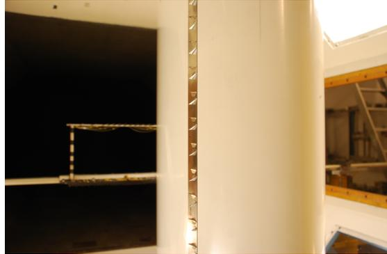
Figure 6.8: Vortex generators installed on airfoil model
