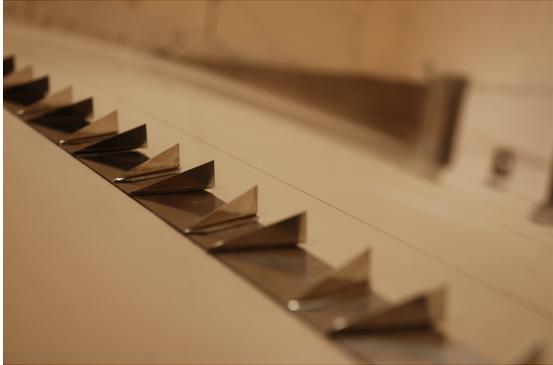
Figure 6.7: Details of vortex generator strip
