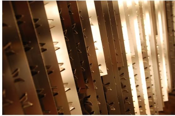
Figure 6.6: Strip of vortex generators with different configurations
