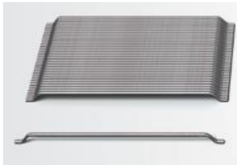
Figure 2.12: Steel fibres with hooked ends [20]
