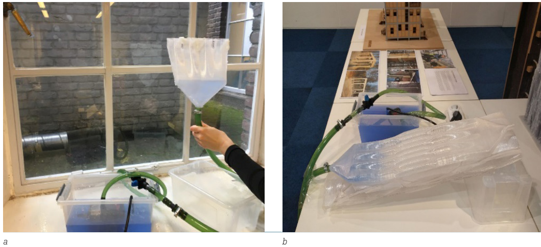
FIG. 5 Water circulation test in the external layer
