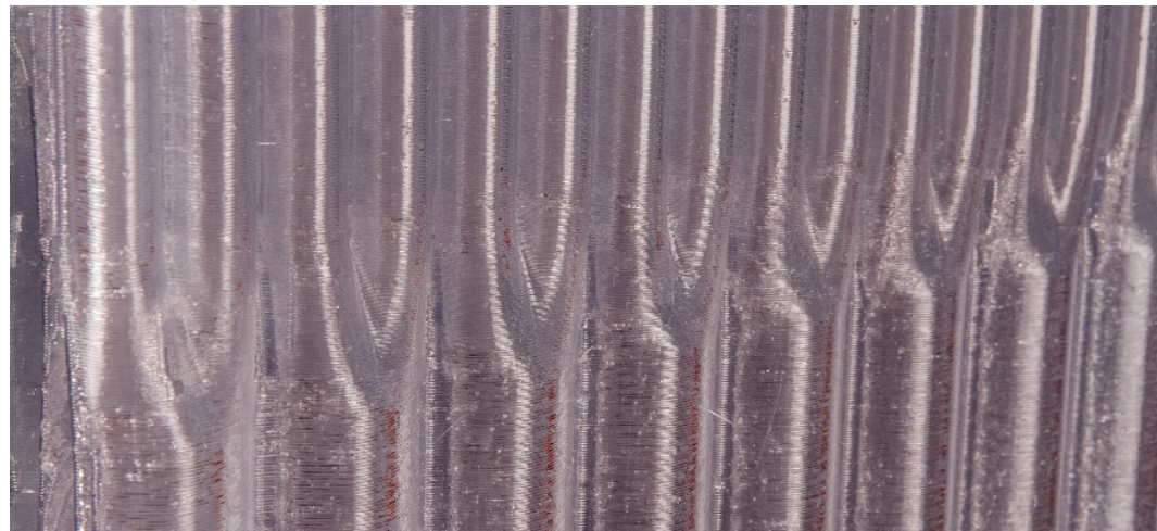
FIG. 4 Printed segment of the external layer
