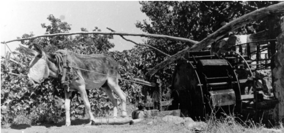
Mechanical system driven by cow or donkey to deliver groundwater from shallow wells. (Ministry of Agriculture, Rural Development and Environment, 2018)
