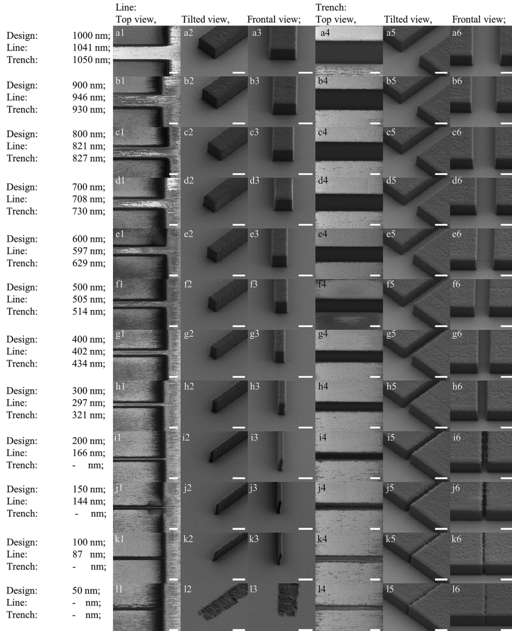
FIG. 5. Micrographs of patterned resist structures fabricated with settings as used for our final fabrication route. Columns: (1)–(3): line patterns and (4)–(6): patterns of trench features. Rows (a)–(l) depict varying design widths. The scale bar has a reference 500 nm length. There is no electrolyte on the resist. The width of the structures is determined with ProSEM and has a standard deviation of 5 nm at 30 000 \times magnification. The 50 nm line has toppled over. Trenches of 200 nm and smaller are underdeveloped. We expect that creating smaller structures can be achieved by tuning the combination of resist thickness, processing bias correction, exposure dose, and development time.
