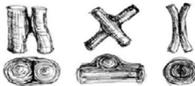
Figure 9 Typical nodes for interconnected trees: Three natural node types are studied: parallel-surface, crosswise and parallel-pith (Nuijten, 2011)
