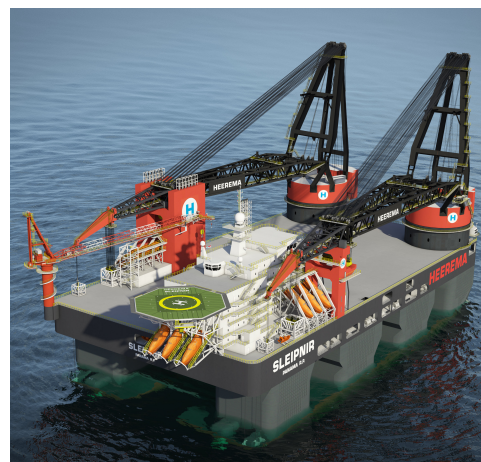
Figure 1: Artist impression of the Sleipnir. A semi-submersible crane vessel with eight columns.
