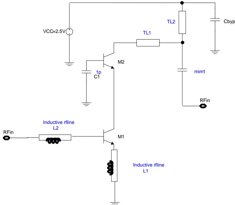
Figure 3.28 single stage inductive degeneration LNA
