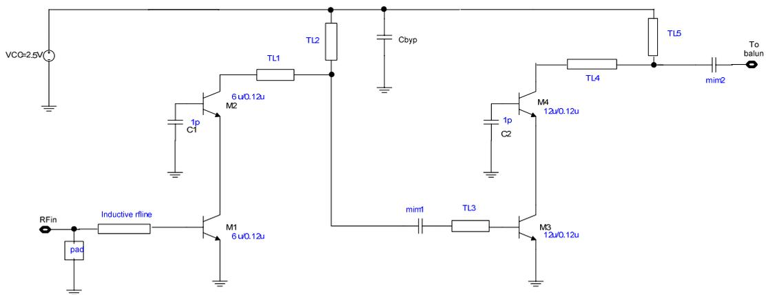
Figure 3.12 schematic of the two-stage cascaded cascode LNA
