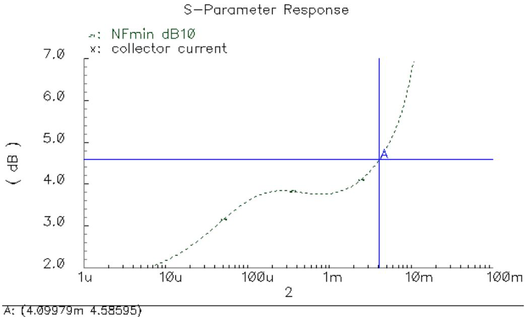
**Figure 3.8 NFmin vs collector current of single transistor**
