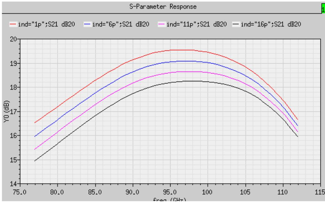
Figure 6.19 S21 variation with the emitter parasitic inductance value
