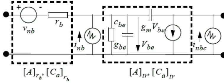
**Figure 3.3 the common-emitter equivalent small signal circuit (base resistance included)**
