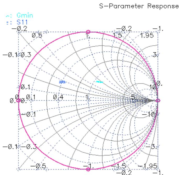
**Figure 3.33 the  $S_{11}$  and  $S_{opt}$  of common-base configuration**
