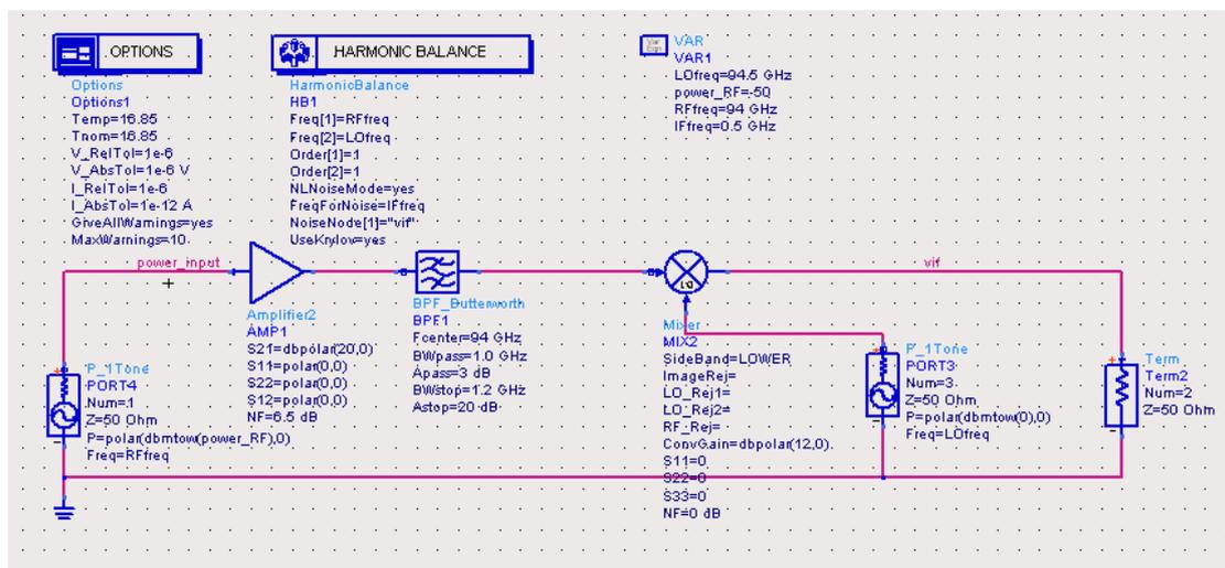
Figure 5.11 an image filter is inserted into the system
