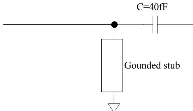
**Figure 6.8 simple high pass filter at the input of LNA**
