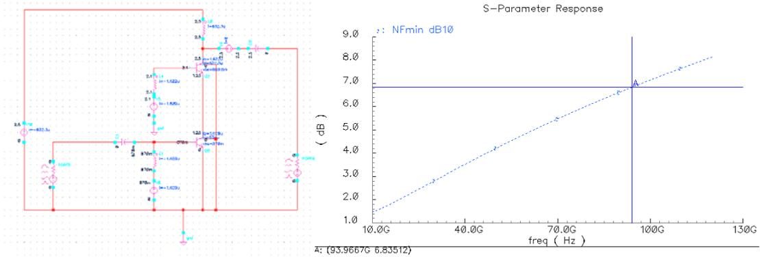
Figure 3.11 NFmin of a cascode stage
