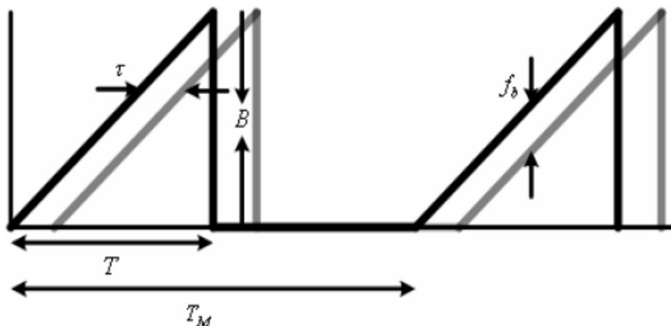
Figure 1.2 modulation scheme for FM-CW radar
