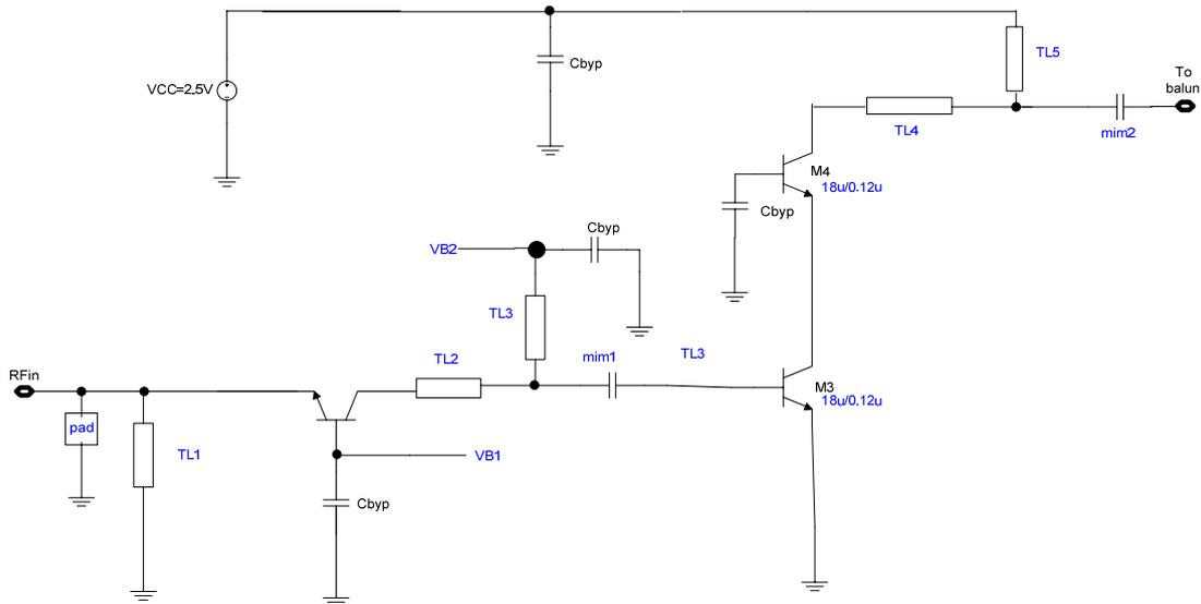
Figure 3.34 the schematic for the common-base input LNA
