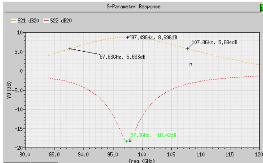
Figure 3.30 S22 and S21 of the single stage LNA
