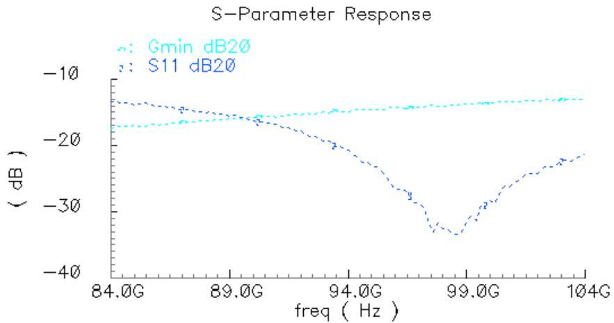
Figure 3.29 simultaneous impedance and noise matching at input port
