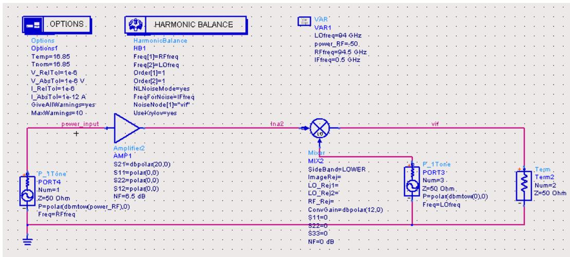
Figure 5.9 system verification by ADS
