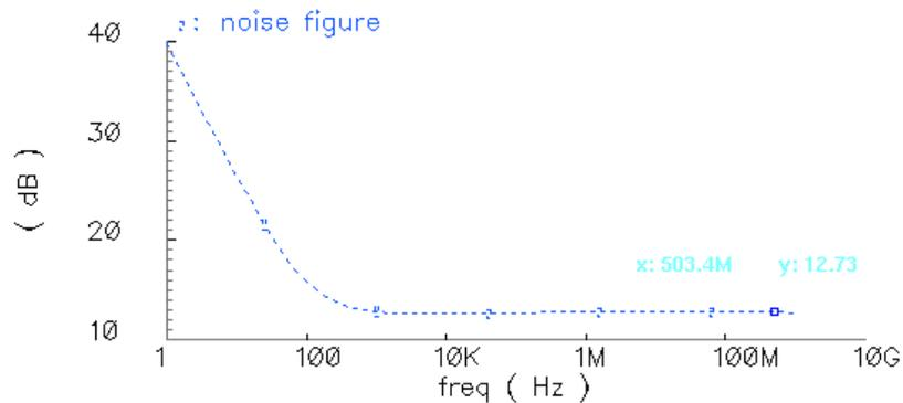
Figure 4.13 noise figure of the dc-coupled-output-buffer mixer
