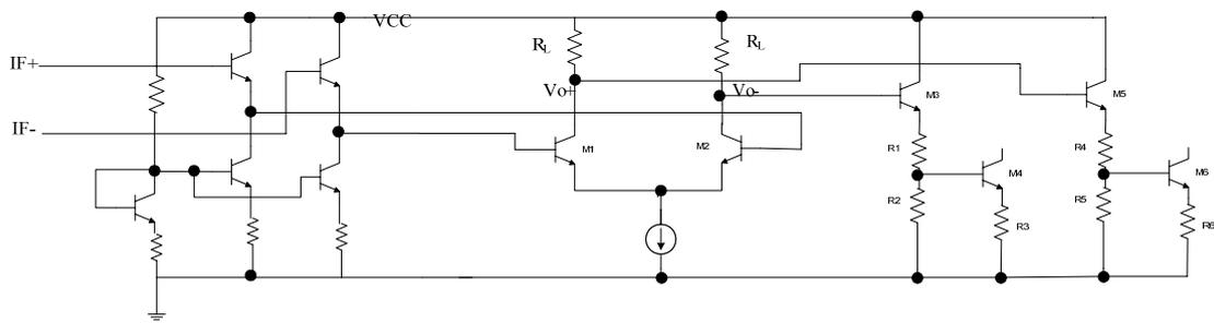
**Figure 4.17** Open collector current adder
