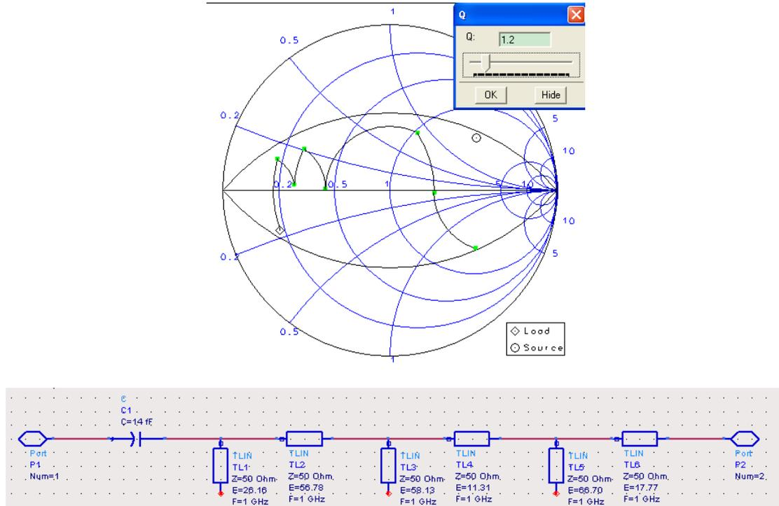
**Figure 3.24 low Q inter stage matching network**
