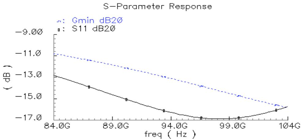
**Figure 3.14 simultaneous impedance matching and noise matching at the input for the first stage**
