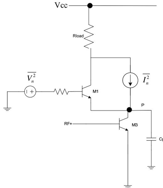
**Figure 4.4 noise contribution by the one of the collector current of the switching pair**
