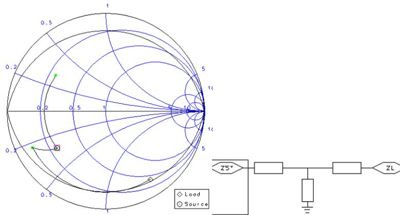
**Figure 3.16 interstage matching principle**
