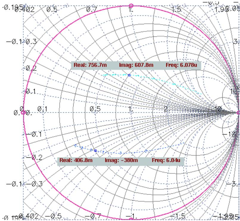
**Figure 3.13 the Gmin and S11 with the length scaling of the first cascode stage**
