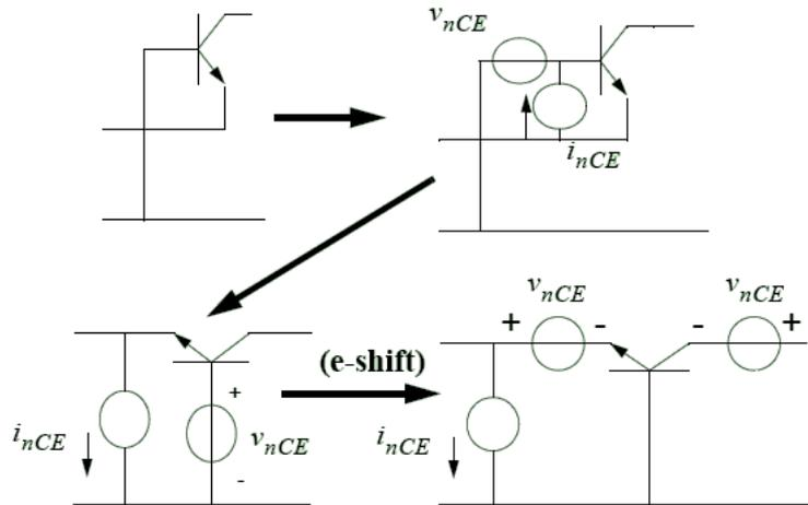
**Figure 3.4 noise transformation of Common base stage**
