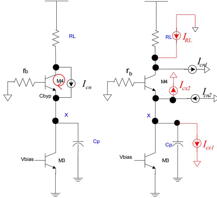
Figure 3.6  $\overline{I_{cn}^2}$  noise analysis
