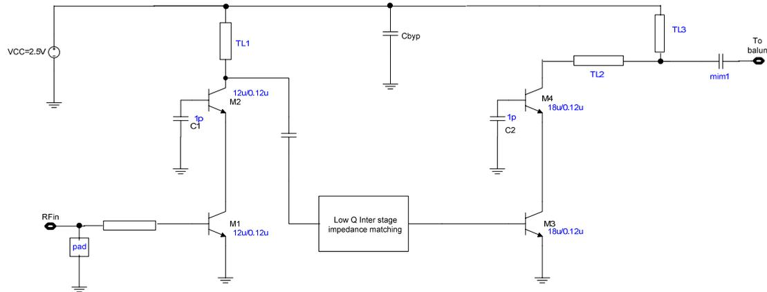
**Figure 3.23 the structure of LNA stage**
