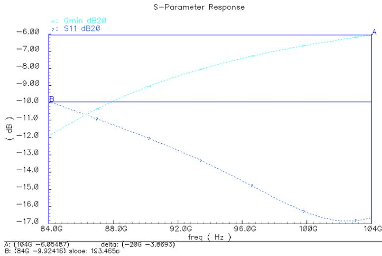
Figure 3.35 impedance matching and noise matching
