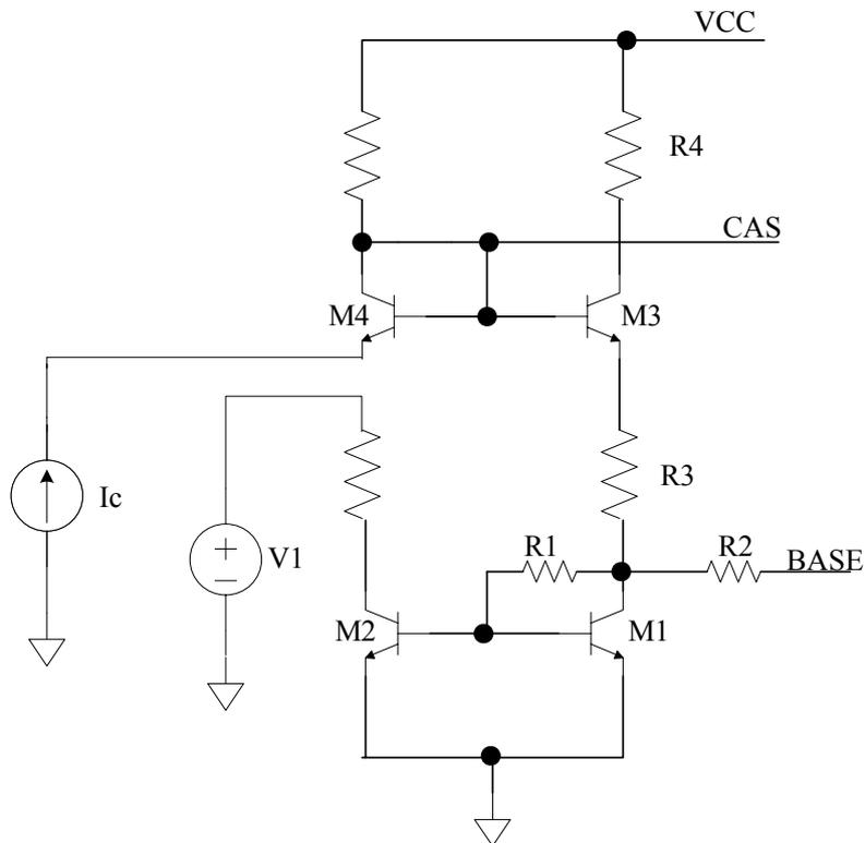
Figure 6.2 ac simulation schematic for the bias circuit
