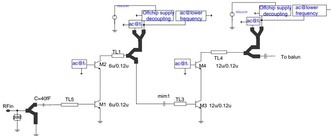
**Figure 6.9 LNA including high pass filter, off chip supply decoupling, and ac ground for  $f_0$  and lower frequencies**
