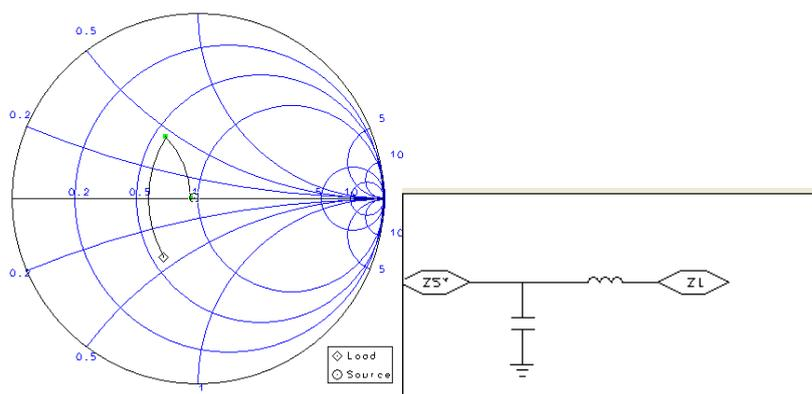
**Figure 3.15 Input matching principle**
