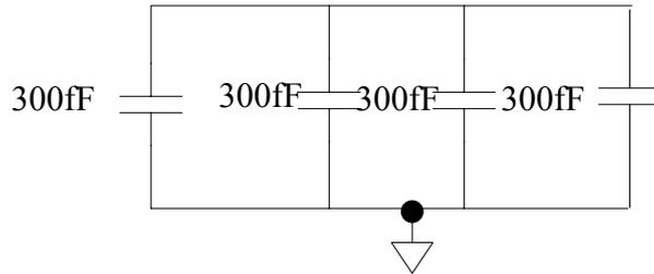
**Figure 6.7 ac ground @ lower frequency**
