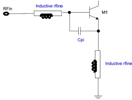
**Figure 3.27 resistive termination by inductive degeneration**
