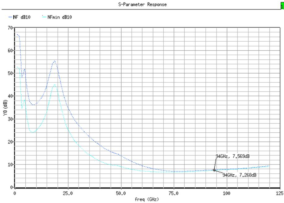
Figure 6.13 NFmin and NF of the LNA
