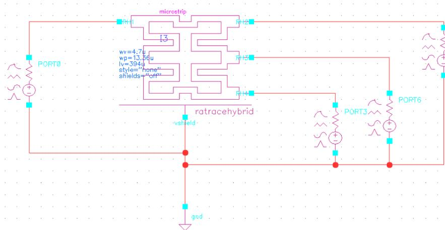
Figure 5.1 schematic for the simulation of the balun
