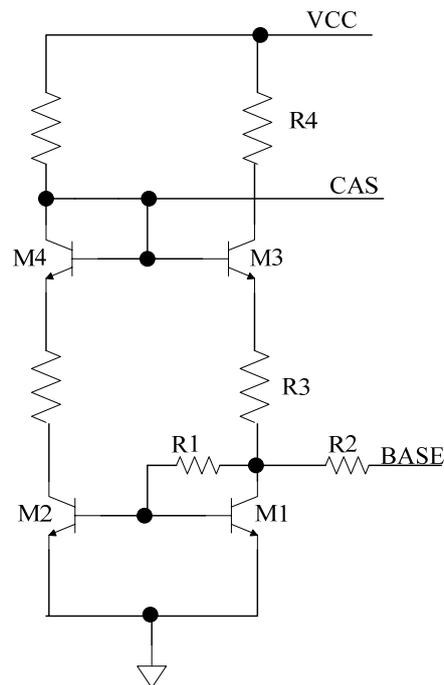
**Figure 6.1 bias circuits for the LNA**
