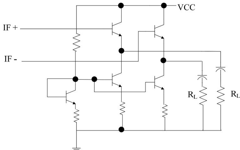
**Figure 4.14 AC coupled output buffer**
