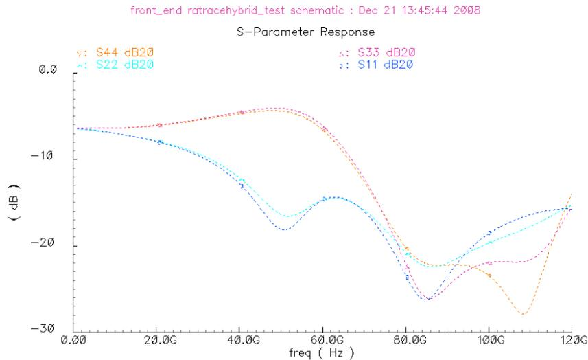
**Figure 5.2 reflection coefficients at each port of the balun**
