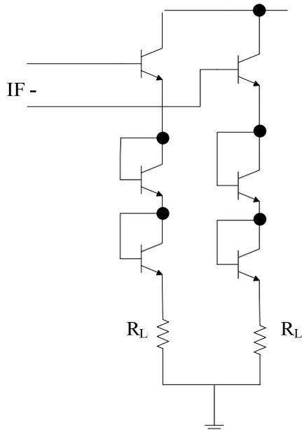
**Figure 4.15 DC coupled output buffer**
