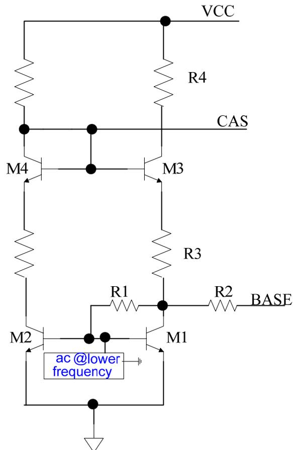
**Figure 6.10 bypass capacitor ac@lower frequency added at the bias circuit**
