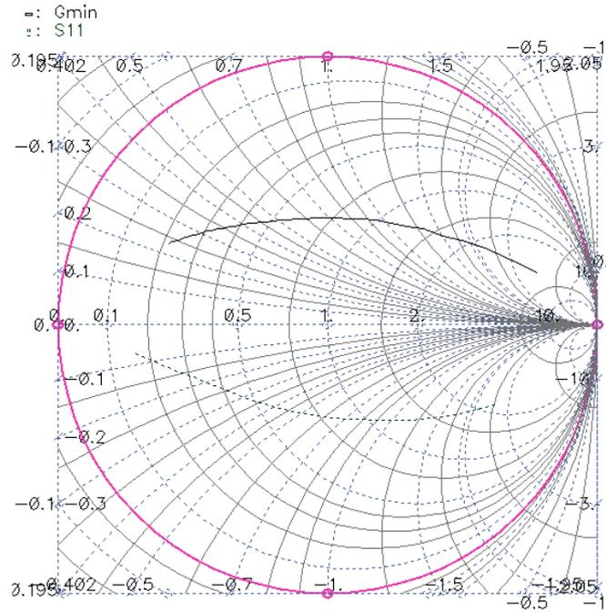
**Figure 3.10 Sopt and S11 of the bipolar transistor vs length in Smith Chart**
