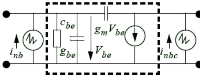
Figure 3.2 the common-emitter equivalent small signal circuit
