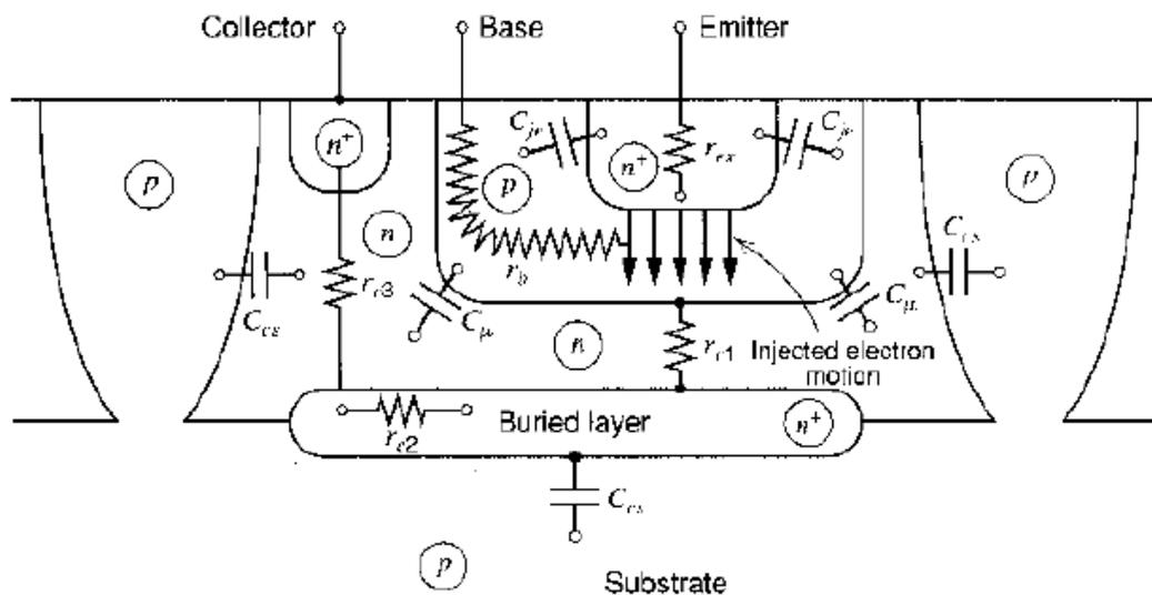
Figure 3.1 integrated circuit npn bipolar transistor structure showing parasitic elements
