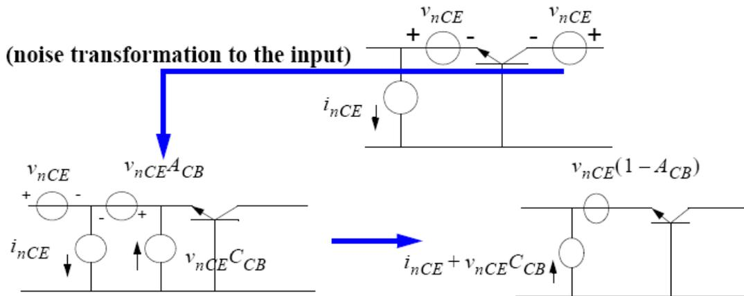
**Figure 3.5 noise transformation of Common base stage**
