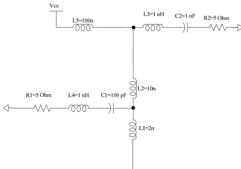
Figure 6.5 off chip supply decoupling network
