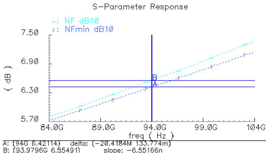
Figure 3.31 NFmin and NF for the single stage
