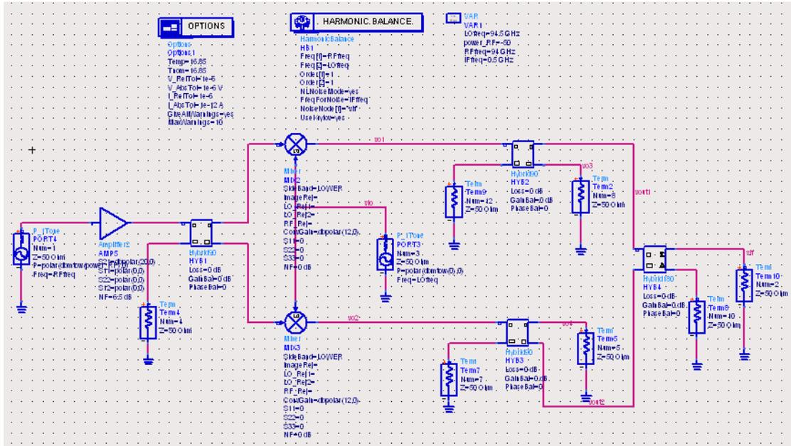
**Figure 7.2 systematic simulation of single side band mixer in the LNA mixer chain**
