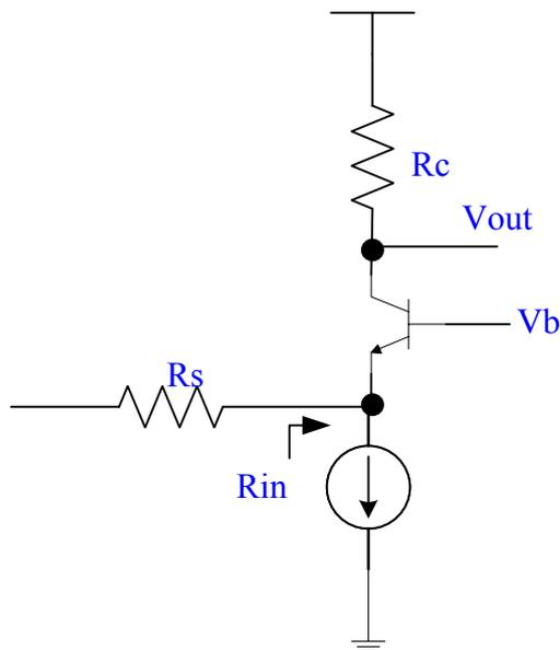
**Figure 3.32 Common-base LNA**
