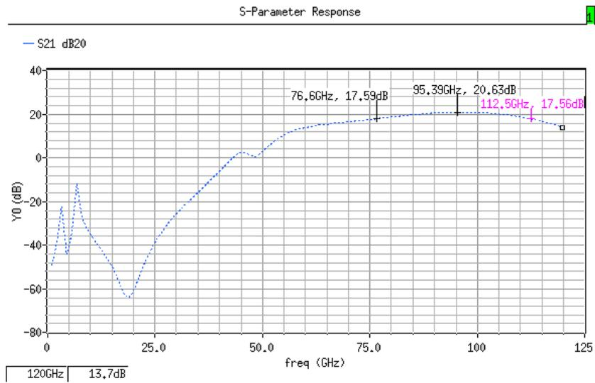
**Figure 6.11 3dB bandwidth throughout 77GHz-112GHz**
