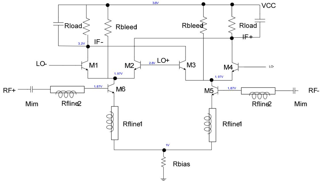
Figure 4.6 the schematic of the double balanced mixer
