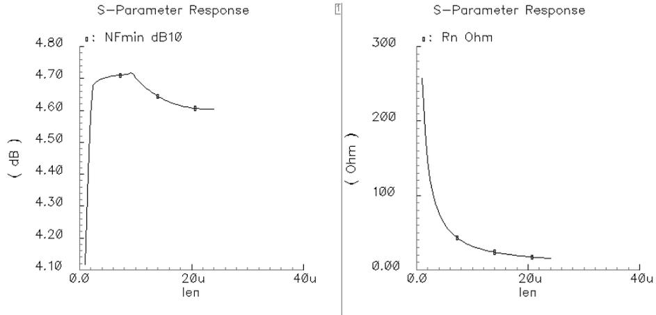
**Figure 3.9 NFmin and noise resistance vs length of the bipolar transistor**
