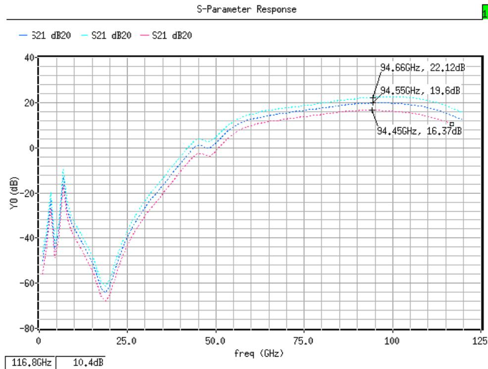
Figure 6.15 process variation of the LNA
