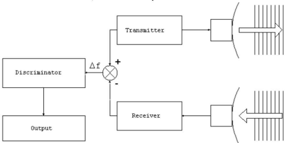
Fig. 1.1 The FM-CW radar principle
