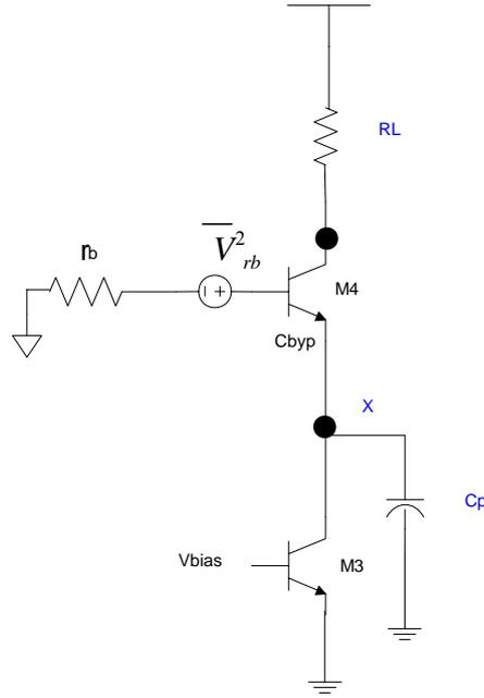
**Figure 3.8**  $\overline{V_{n,rb}^2}$  noise analysis
