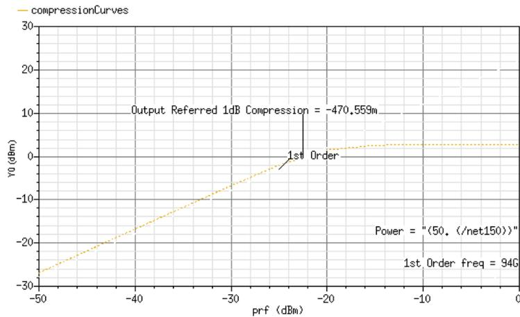
Figure 3.20 1dB output compression point of LNA
