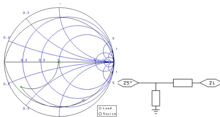
**Figure 3.17 Output impedance matching principle**
