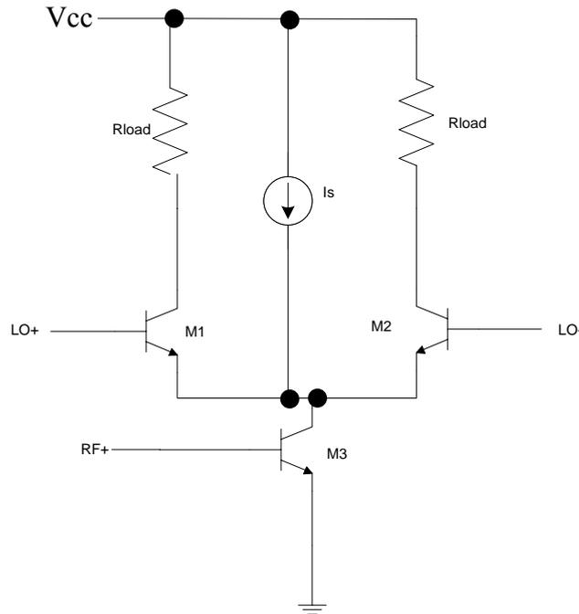
Figure 4.5 current bleeding by  $I_s$  to reduce noise
