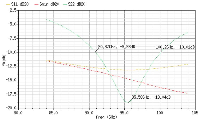
**Figure 3.18 S11,S22, Gmin of the two stage cascaded cascode LNA**
