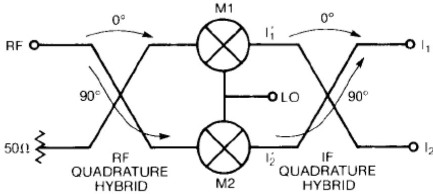
**Figure 7.1 Block diagram of a single-sideband mixer**
