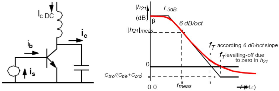
**Fig 3.6 is the schematic for testing the  $f_T$  of a single transistor**
