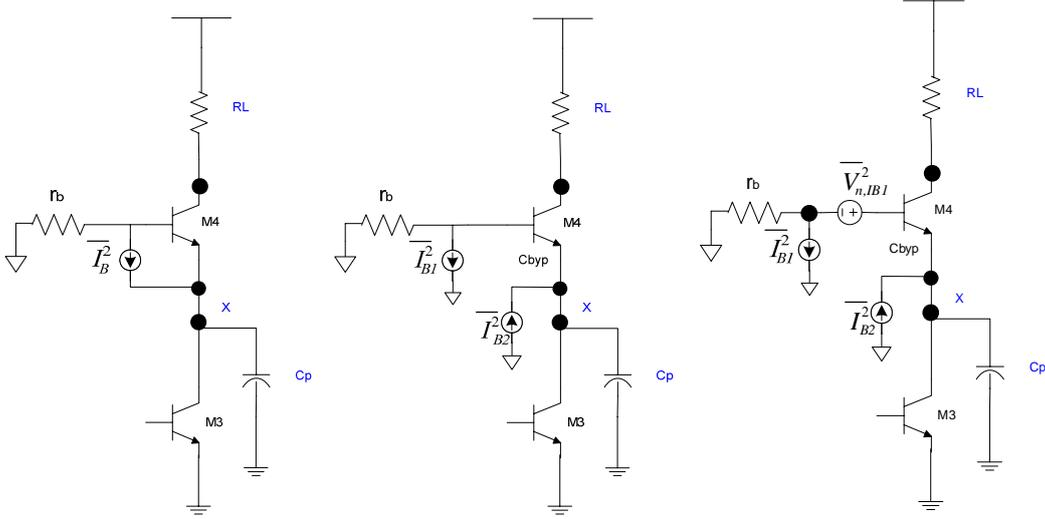
Figure 3.7  $\overline{I_{bn}^2}$  noise analysis
