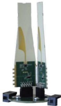
(a) Two antipodal vivaldi antennas used in high frequency board
