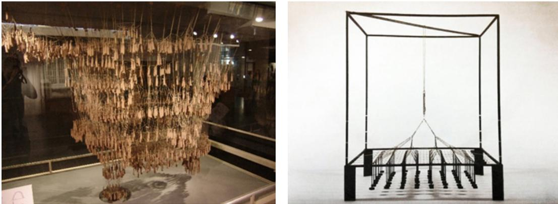
Figure 9 The hanging model of the Sagrada Família (a) and right frei otto's model study (b)
