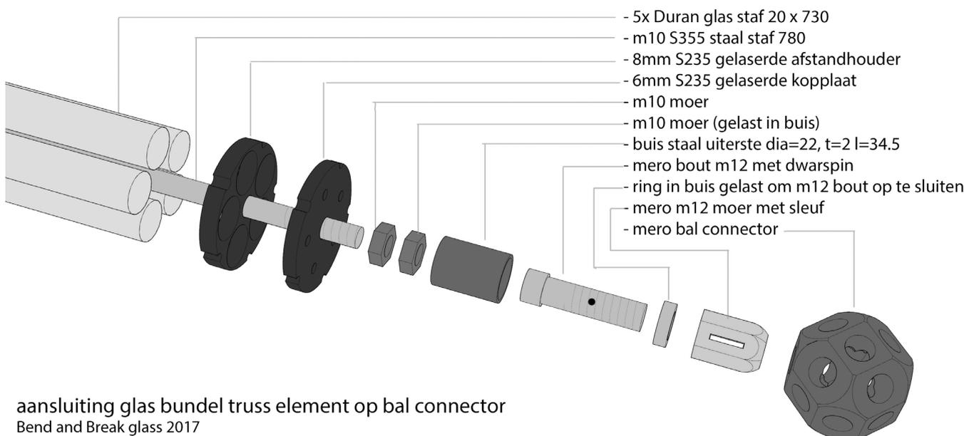
Figure 73 Bundled glass truss element (Bend and break, TU delft)
