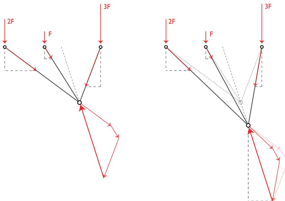
Figure 47 Scaling the branching point along working line (Own image)
