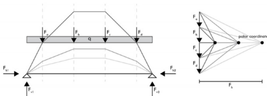
Figure 16 Different thrust lines for different polar coordinates (Dool, 2012)
