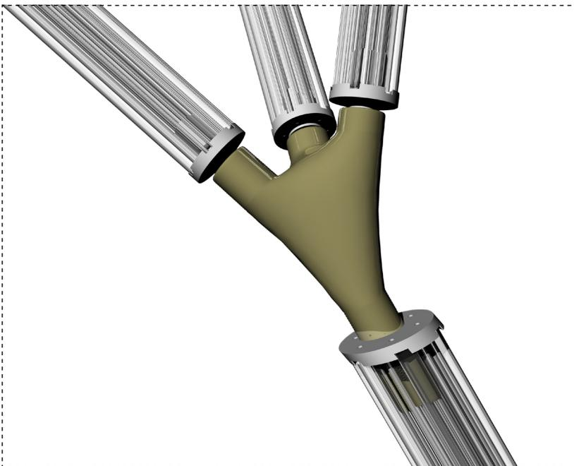
Figure 82 Detailed (3D printed) connection (Own image)
