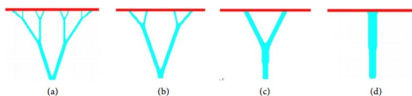
Figure 12 Increasing stiffness of the roof element leads to different optimal shapes (Peng, 2016)
