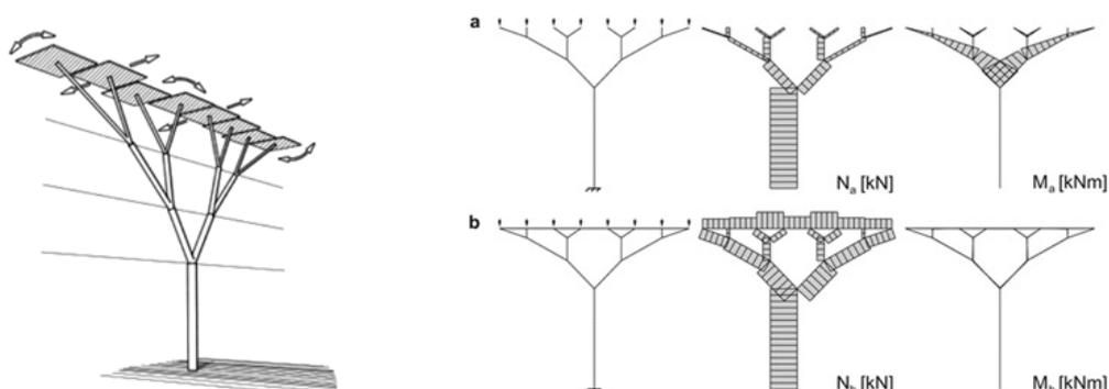
Figure 7 Free moving branches of a real tree (a) and comparison of structural behavior (b) (Zhao et al., 2017)
