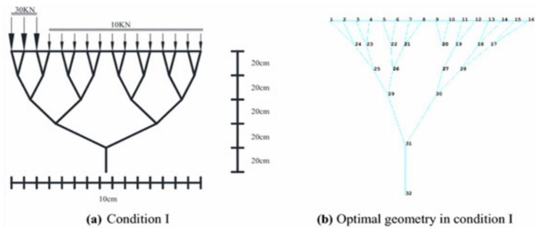
Figure 11 form-finding of non-uniform distributed loads using double element method. (Zhao et al., 2017)
