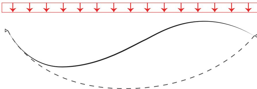
Figure 65 Buckling shape of freeform roof structure (Own image)
