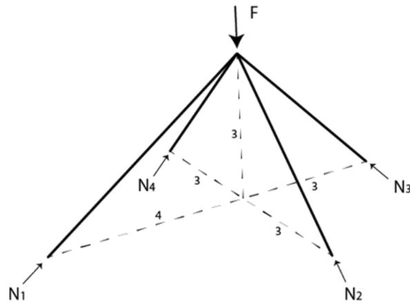
Figure 23 Statically indeterminate system (Own image)
