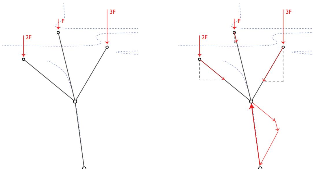
Figure 55 Moving the point to the working line, excluding bending moments (Own image)
