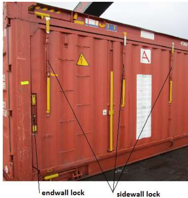
Figure 16 Endwall and sidewall lock details
