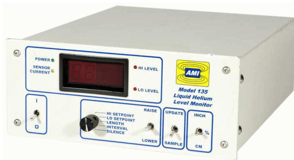
**Figure A.9 Model 135 Liquid Helium Level Monitor**
