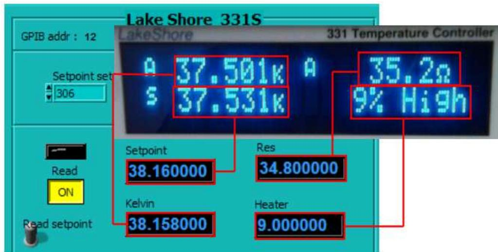
**Figure A.28 Comparison between the Lakeshore 331 Temperature Controller block and front panel during a working measurement.**
