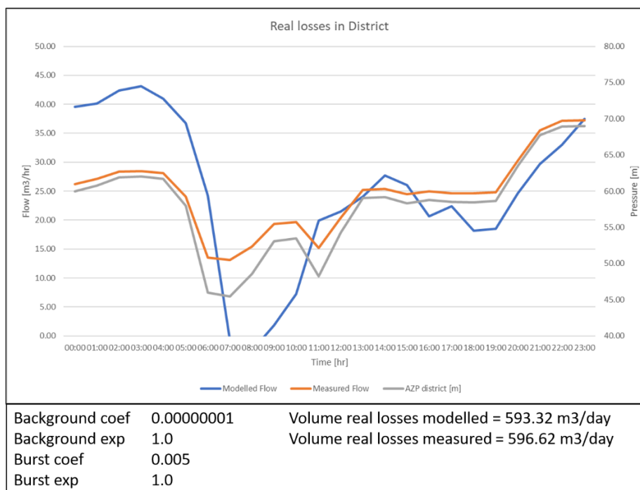
Figure 51 Modelled leakage volume with WaterNetGen.
