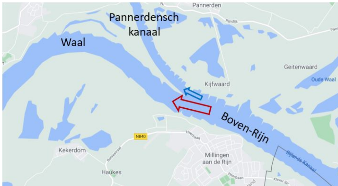
Figure 3.2: The Pannerdense Kop bifurcation. Approximately 2/3 of the discharge at the river Bovenrijn flows into the river Waal, indicated by the red arrow. The remainder of the water flows into the river Pannerdensch Kanaal, indicated by the blue arrow.
