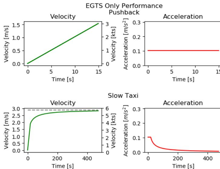
Figure 5.14: Performance of the RETS when only APU power is available.
