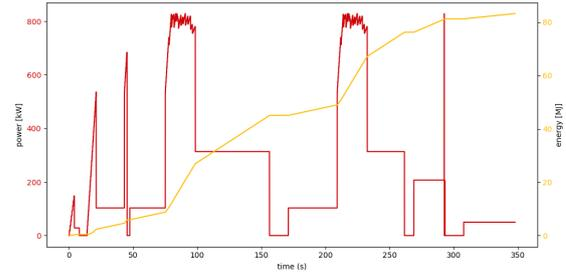
Figure 4.17: Power distribution and cumulative energy consumption for the baseline taxi-out scenario.
