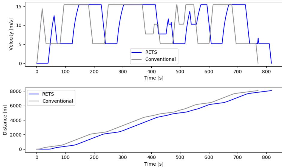
Figure 4.12: Velocity and distance profile for the taxi route Polderbaan to gate D-14.
