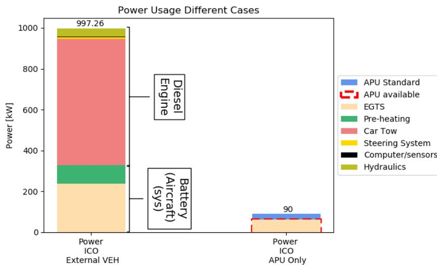
Figure 5.8: Breakdown of (peak) power consumed by RETS
