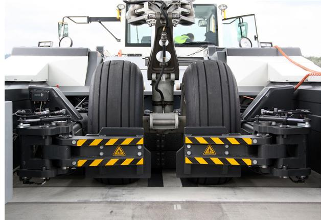
Figure 6.6: Goldhofer Phoenix AST-2X Lifting Cradle <sup>89</sup>
