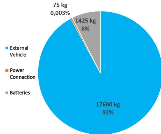
Figure 3.2: Nose wheel vehicle mass budget
