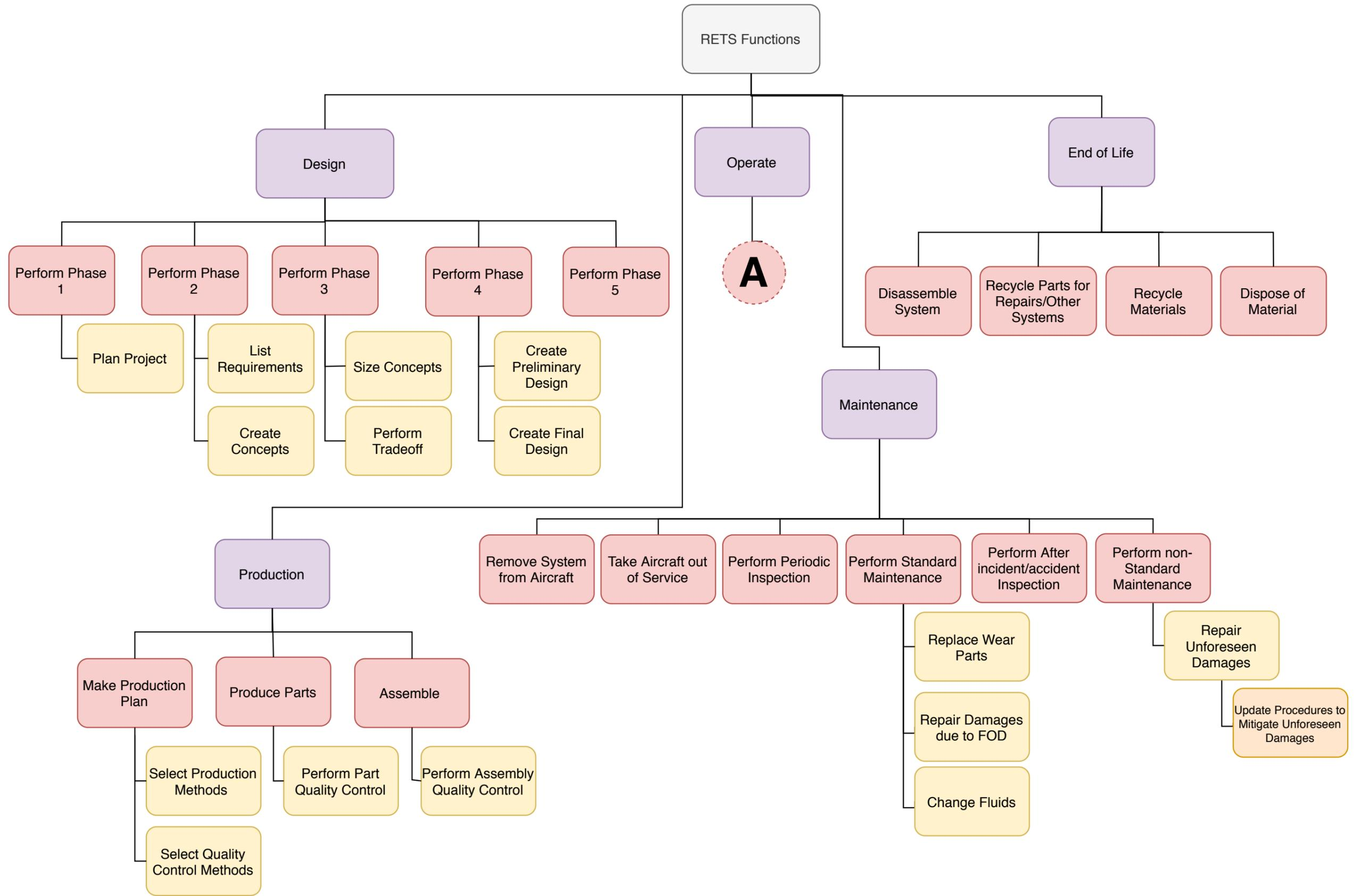
Figure 4.4: General functional breakdown structure taken from Baseline Report [3]
