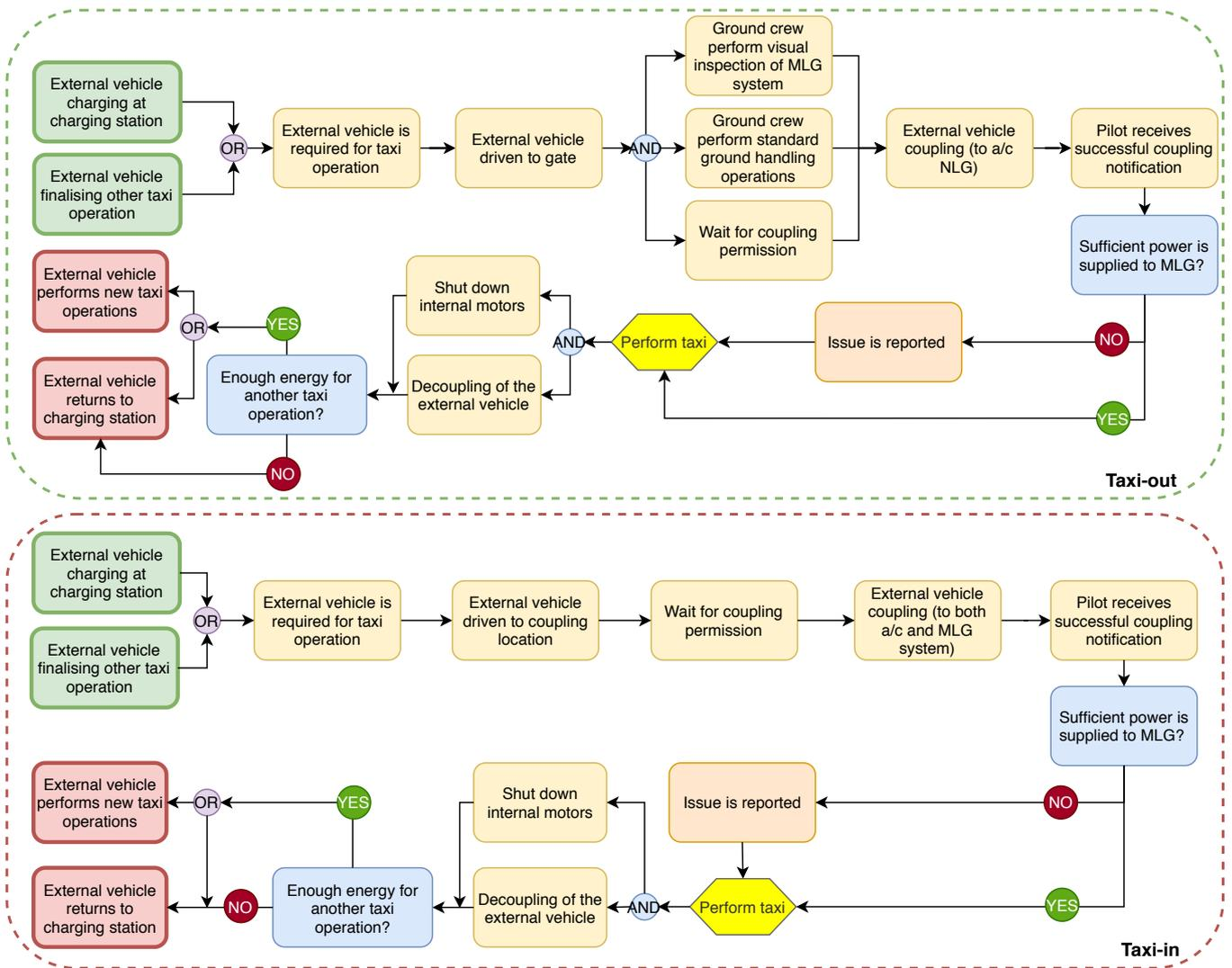
Figure 4.2: Taxi-in & Taxi-out Functional Flow Diagrams based on [1]
