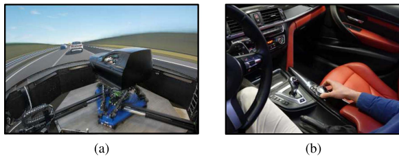
Fig. 4. Experiment setup (photos adapted from [16]). (a) Ruby Space simulator while moving. (b) Test driver using the rating knob.
