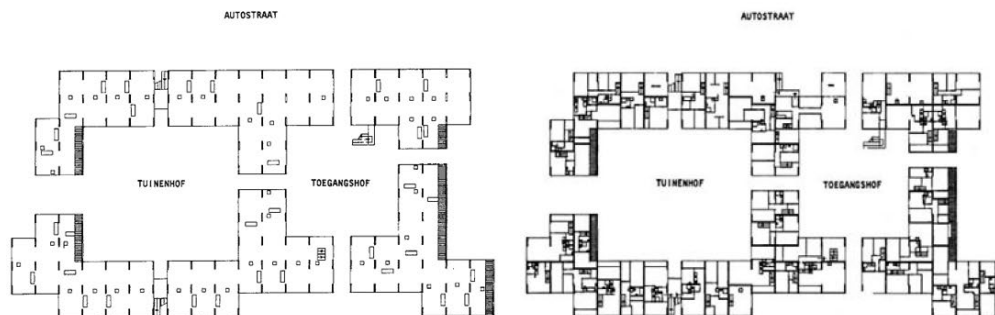
Floor plan of bare support (left) and floor plan after parcellation and infill (right), by Frans van der Werf, from: Kendall and Teicher, 2002, p. 94
