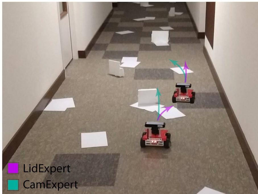
Figure F.3: The robot encounters the first obstacle. The actions predicted by both the LidExpert and CamExpert are visualized.
