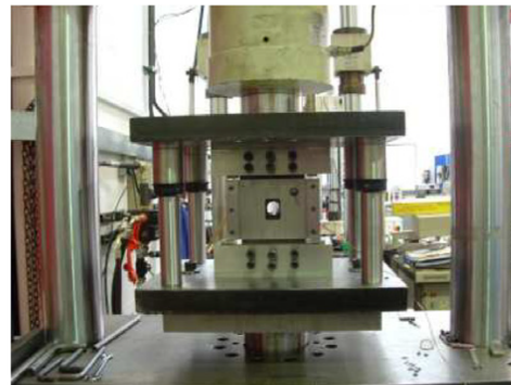
Figure A.3: ICSTM test fixture [39]
