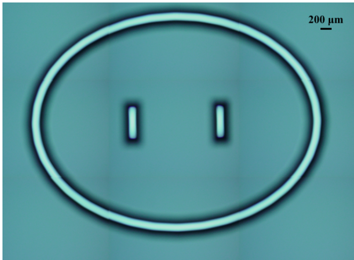
Figure 3.25: Micropillar oxide mask after etching.
