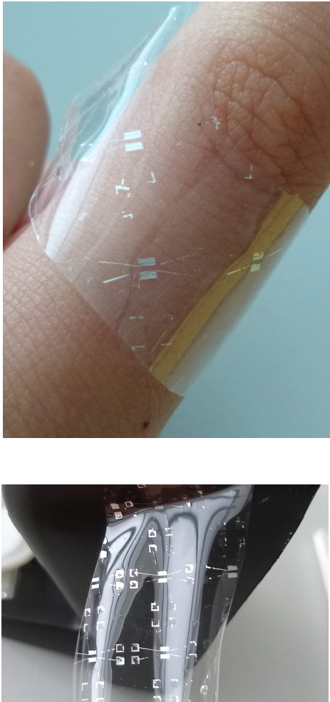
Figure 3.23: Partial detachment of flexible spiral sensors on peeling of second PDMS layer.
