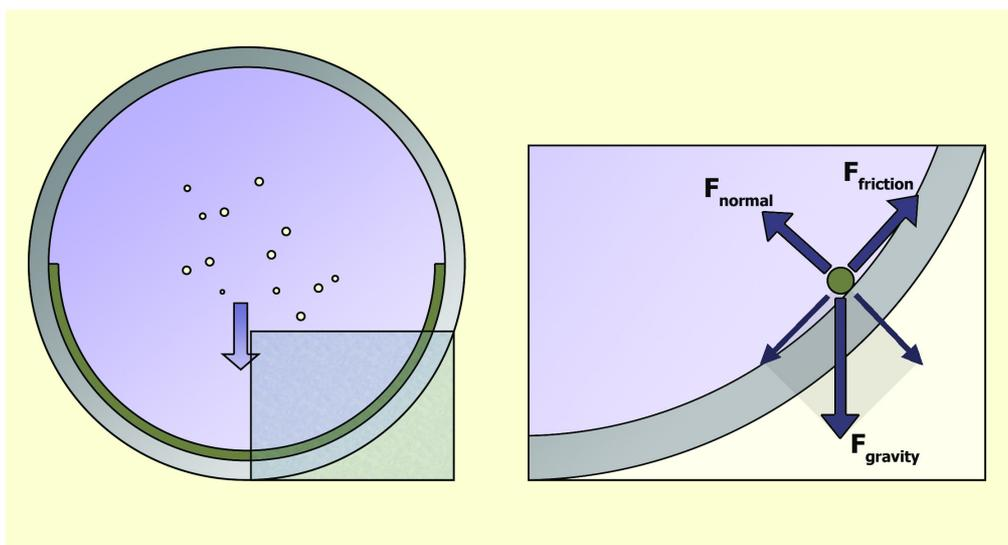
figure 8.26 Force analysis of a particle on the pipe wall
