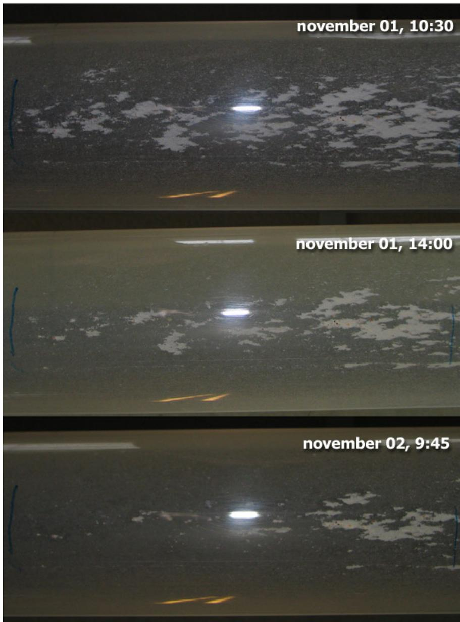
**figure 8.31 Remobilisation of sediment [location1]**
