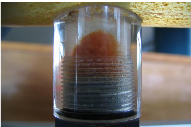
**figure 8.6 Accumulation of sediment resulting from bed load transport**
