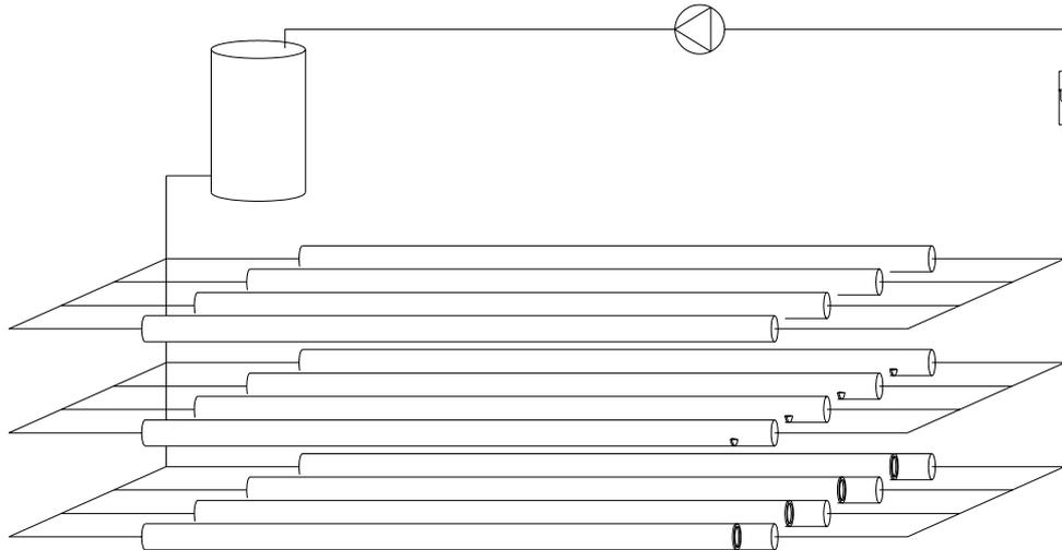
**figure 5.1 Impression of a multiple pipe setup with different kind of wall obstructions**
