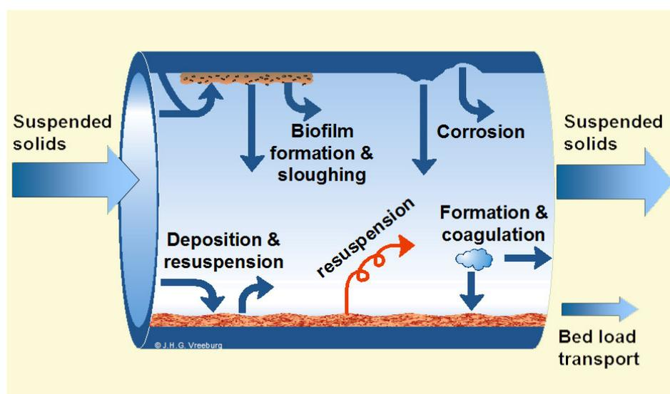
**figure 3.1 Mass balance for a distribution system**
