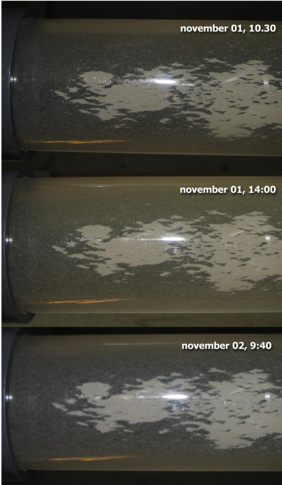
*figure 8.32 Remobilisation of sediment [location2]*
