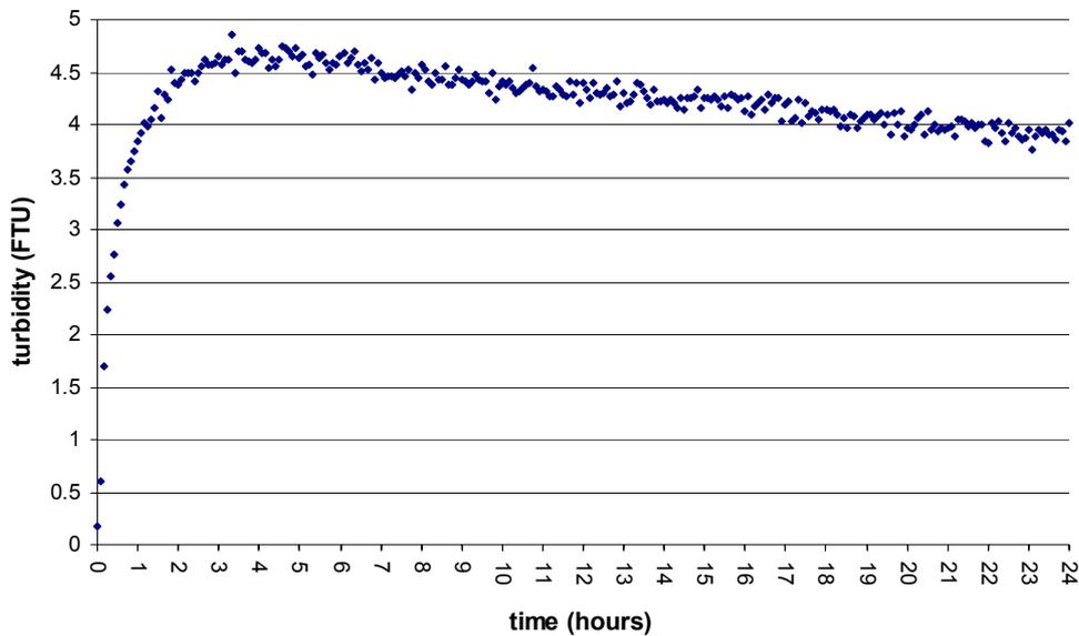
**figure 8.30 Remobilisation of sediment after acceleration of flow velocity**
