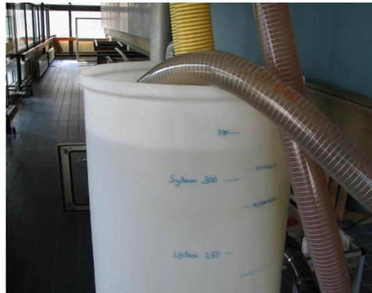
**figure 5.5 Reservoir of the test rig**
