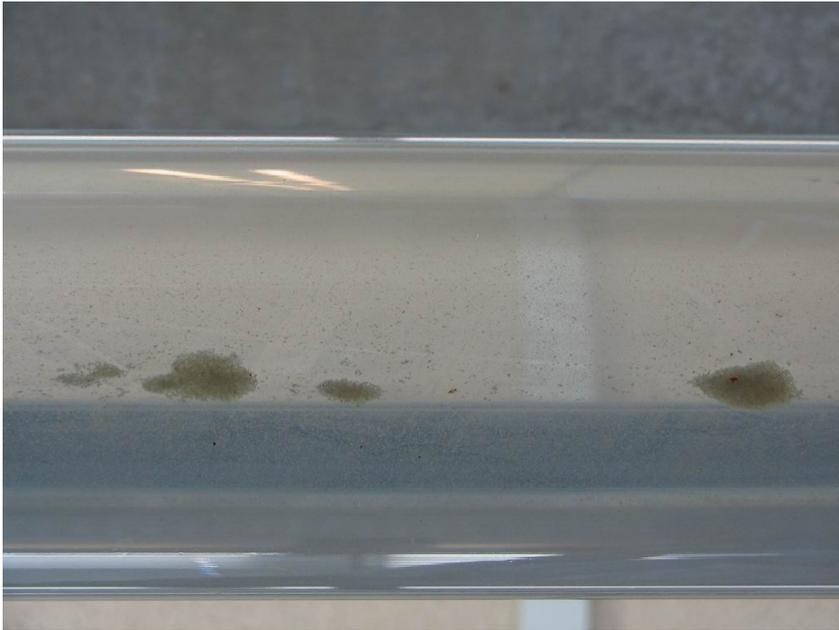
**figure 8.3 Typical accumulation of kaolinite (picture taken from below)**
