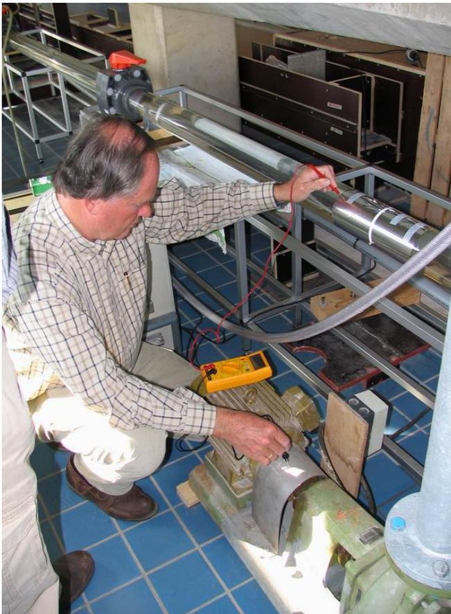
**figure 8.9 Bram v/d Veer looking for electrostatic effects**
