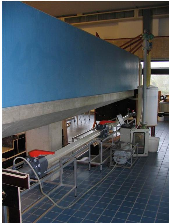
**figure 5.2 Single pipe test rig**
