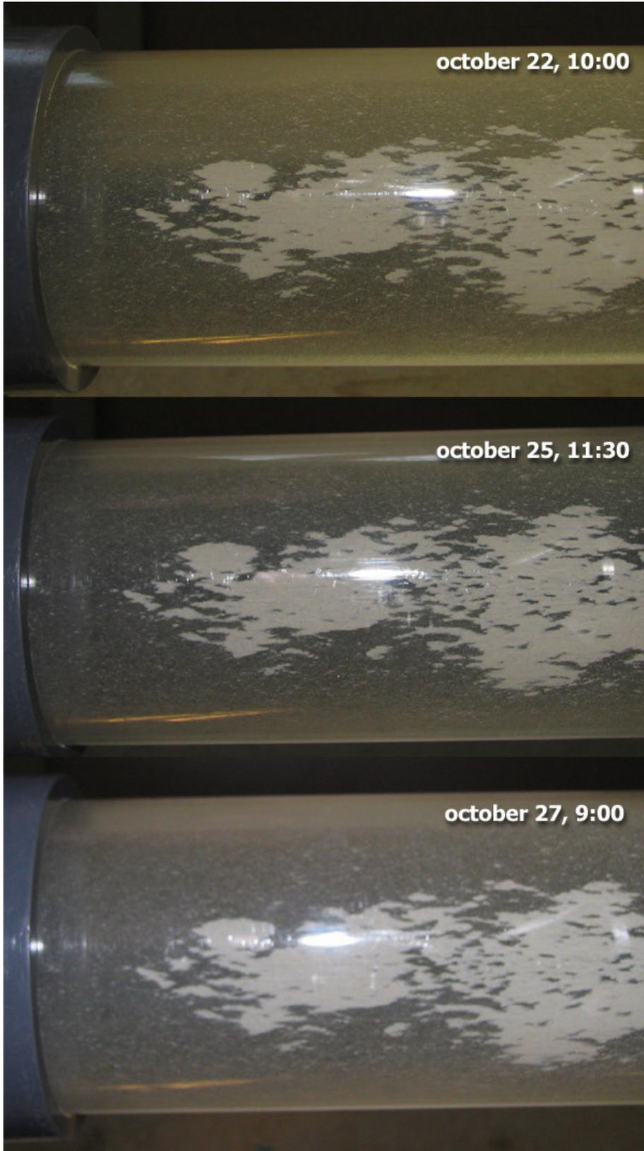
*figure 8.29 Observation of bed load transport [location2]*
