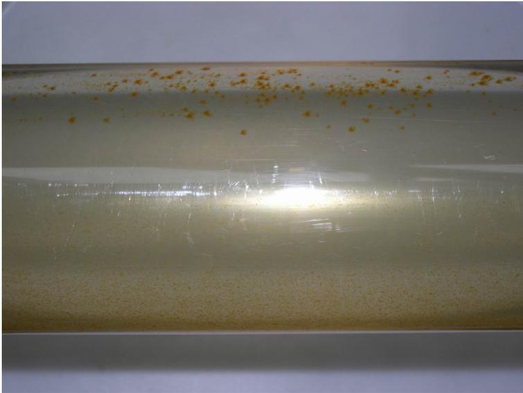
**figure 8.5 Fouling of the top half of the pipe caused by air bubbles (side view)**
