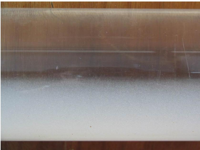
**figure 8.4 Typical layer development with kaolinite (side view)**
