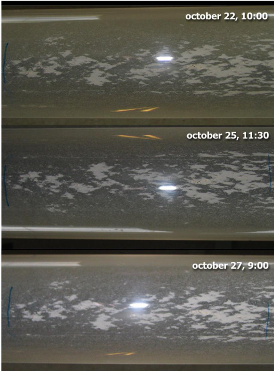
*figure 8.28 Observation of bed load transport [location1]*
