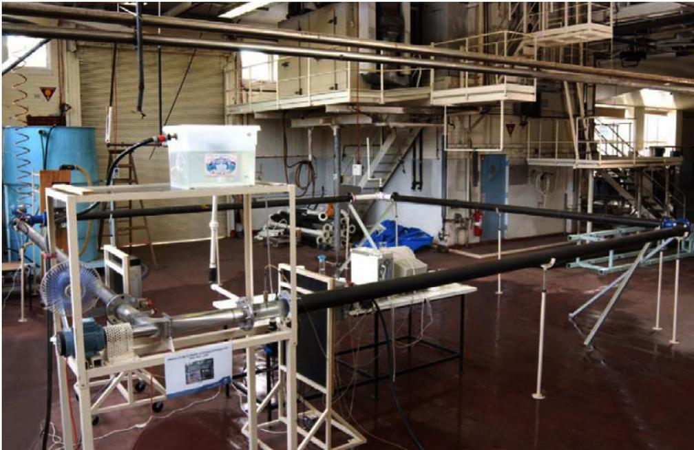
**figure 2.2 Particle sediment test loop (PSTM)**
