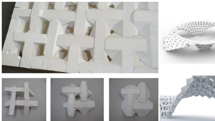
Figure 2.6 The problem of porosity of Type 1 when they are assembled together (Source: Philipp Mecke)
