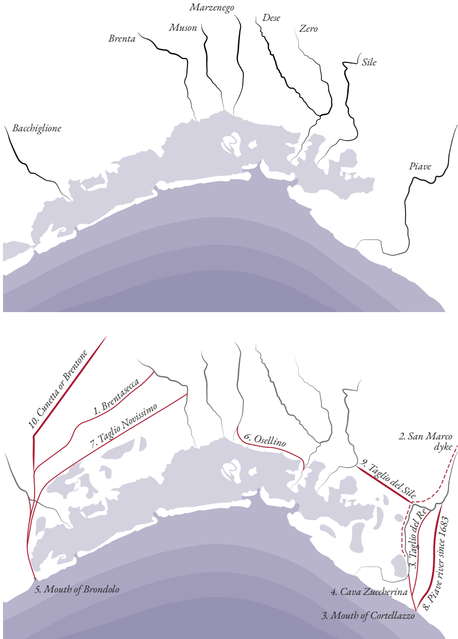
fig. 04/03 SCHEMATIC DIAGRAM OF THE DIVERSION OF RIVERS FROM THE LAGOON (16TH-19TH CENT.)
